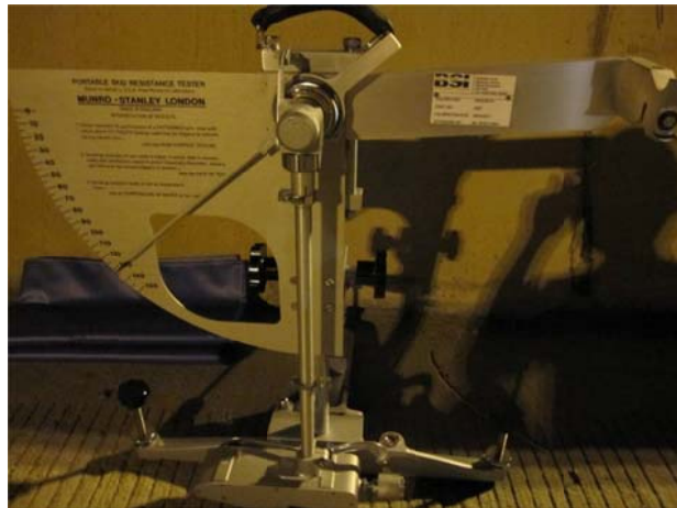
Fig 3.10 British Pendulum Tester
