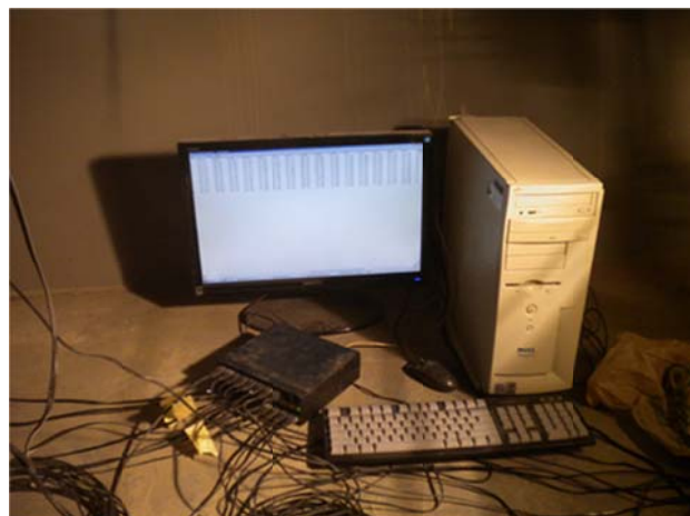
Fig 3.16 The data logger recording data for the integrated sensors
