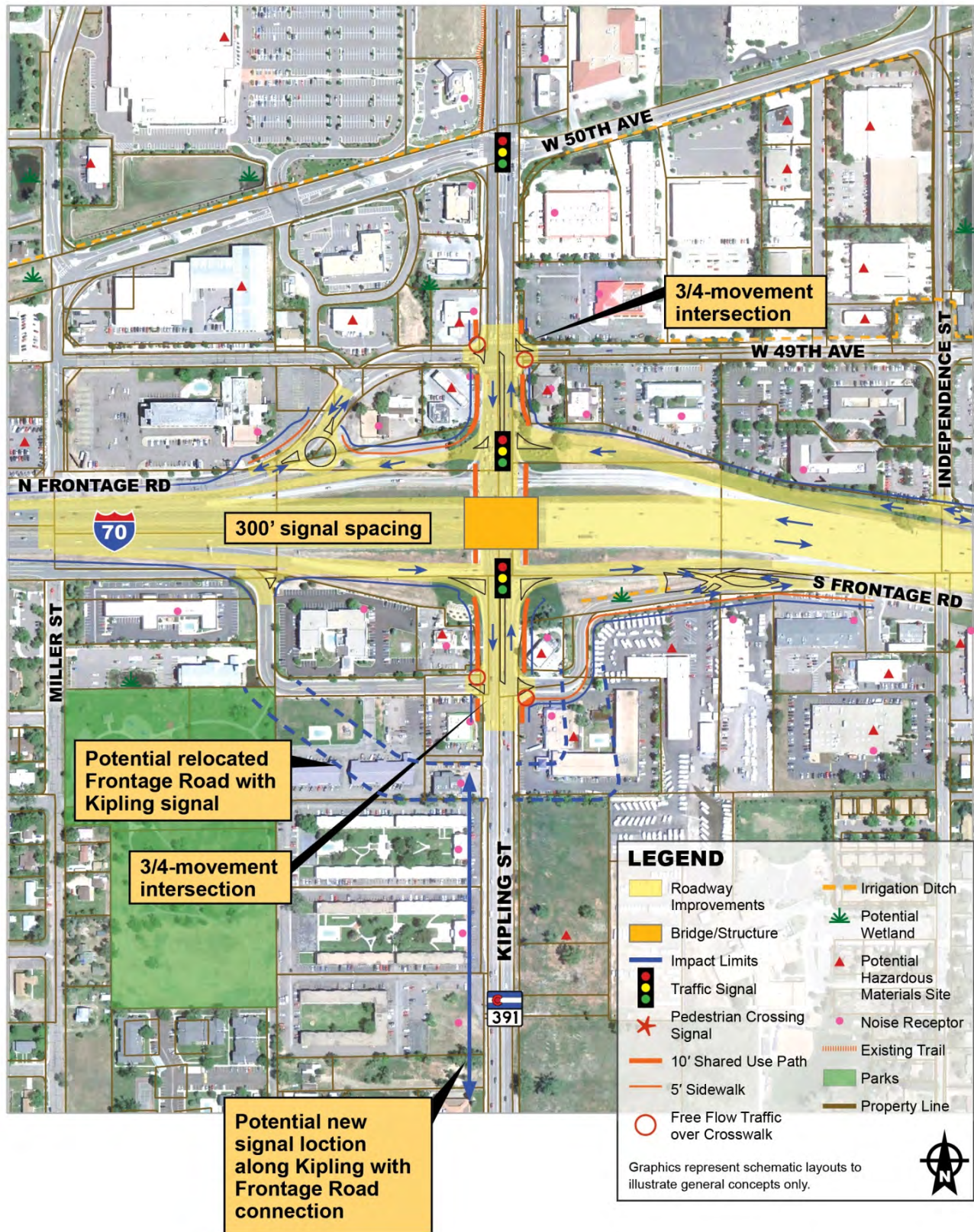
Figure 16: Alternative 11 - Texas Frontage Road Diamond
