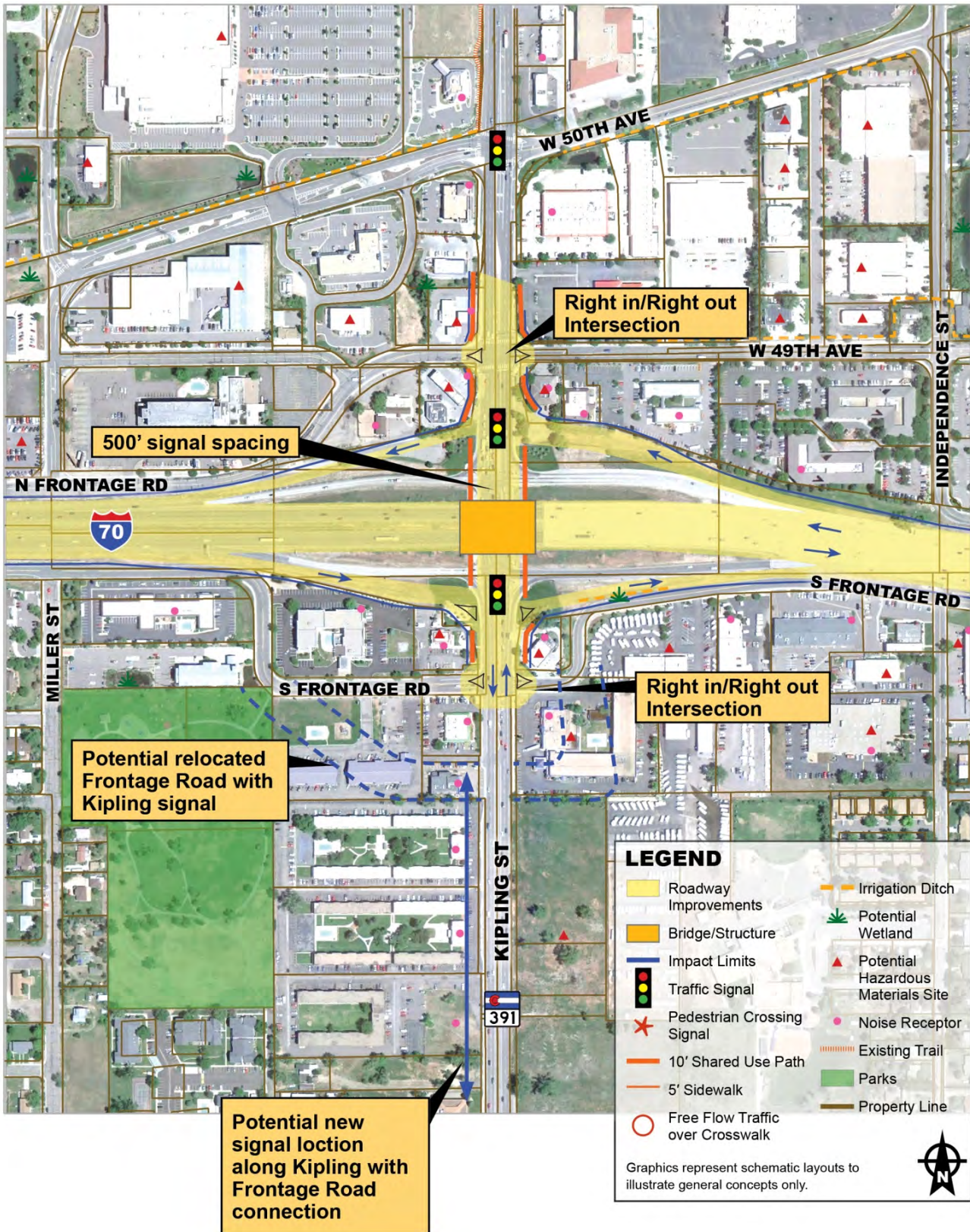
Figure 17: Alternative 12 - Traditional Diamond
