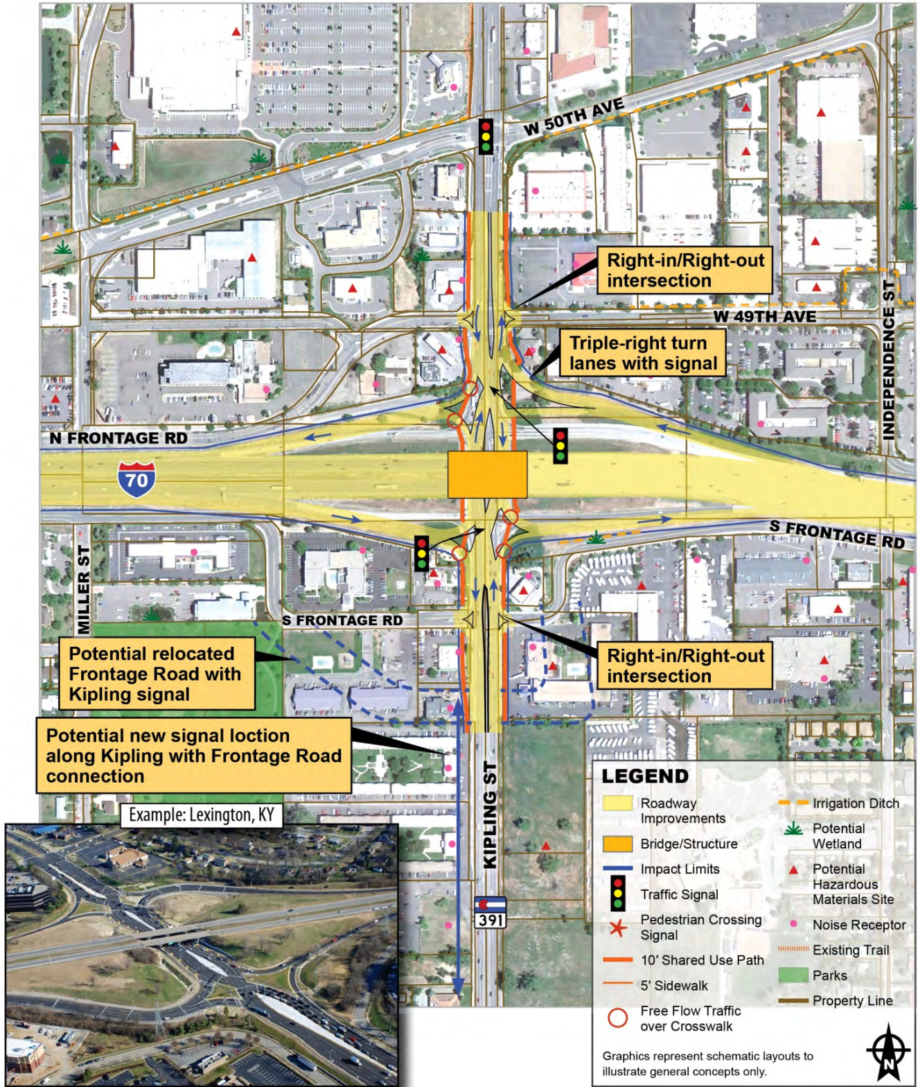
Figure 23: Alternative 35 - Double Crossover Diamond Interchange
