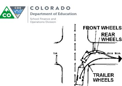
The longer the trailer, the wider you must swing in a turn to make sure the trailer wheels clear the inside curb.
