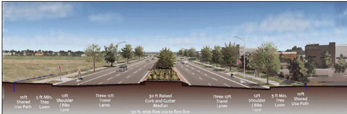
Figure ES.1 Typical Cross-section – Segment 3
