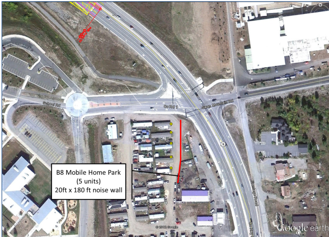
1 Figure 5 Location of B8 Mobile Home Park Noise Wall
