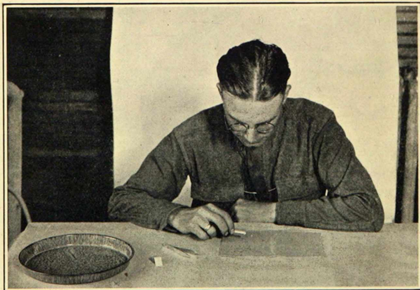
FIGURE 4. Scattering seeds from a small vial on moist blotting paper.
