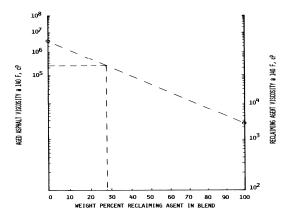
Figure 1, Nomograph for Viscosity.
