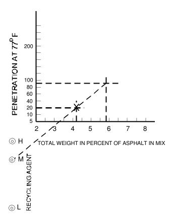
To use: Enter a point, "X", corresponding to asphalt content and penetration in aged pavement. Draw a straight line from the selected origin,(L- low, M-med, H-high) O, through "X". Intersection of this line with a vertical line representing desired asphalt content of recycled pavement (aged asphalt + recycling agent) gives predicted approximate penetration of rejuvenated asphalt.
