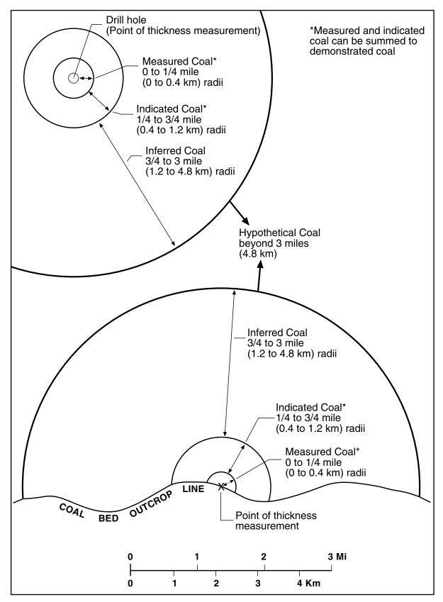
Figure 3. Diagram showing reliability categories base solely on distance from points of measurement (from Wood and others, 1983).
