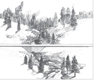
A / Seasonal and ephemeral stream courses can be placed in a culvert for short sections as they cross the corridor. Naturalized channels should be maintained and enhanced on both the uphill and downhill sections as a landscape and visual feature.
