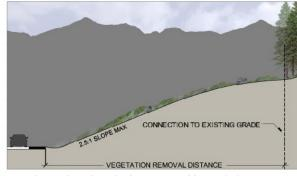
*C* | *The preferred method requires additional clearing to round grading properly, yet creates a more natural slope and vegetation condition.*
