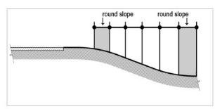
*B* / To transition into existing grade, round the slope over the last one sixth of the top and toe of the embankment.
