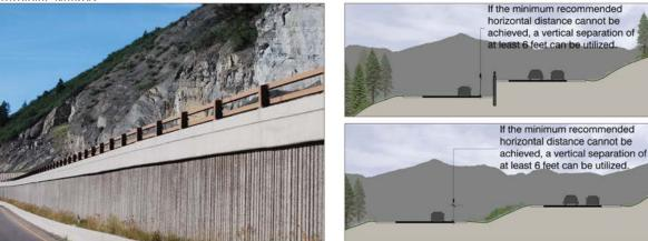
*C* | Where steep topography restricts median width, a vertical separation of at least 6' should be implemented.
