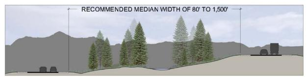
$B \mid A \text{ median of } 80' \text{ to } 1,500' \text{ provides an appropriate separation of the travel lanes and allows space for landscape and hydrologic features}$
