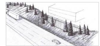
E | Utilize berms and landforms as much as possible to reduce F | Elevation changes on the top of sound walls should the need for exposed sound wall structures.
