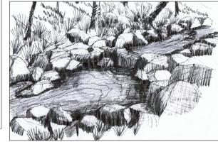
$D \mid Drop \ structure \ using \ indigenous \ rock \ construction.$
