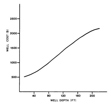
Figure 5. Well costs for groundwater wells.
