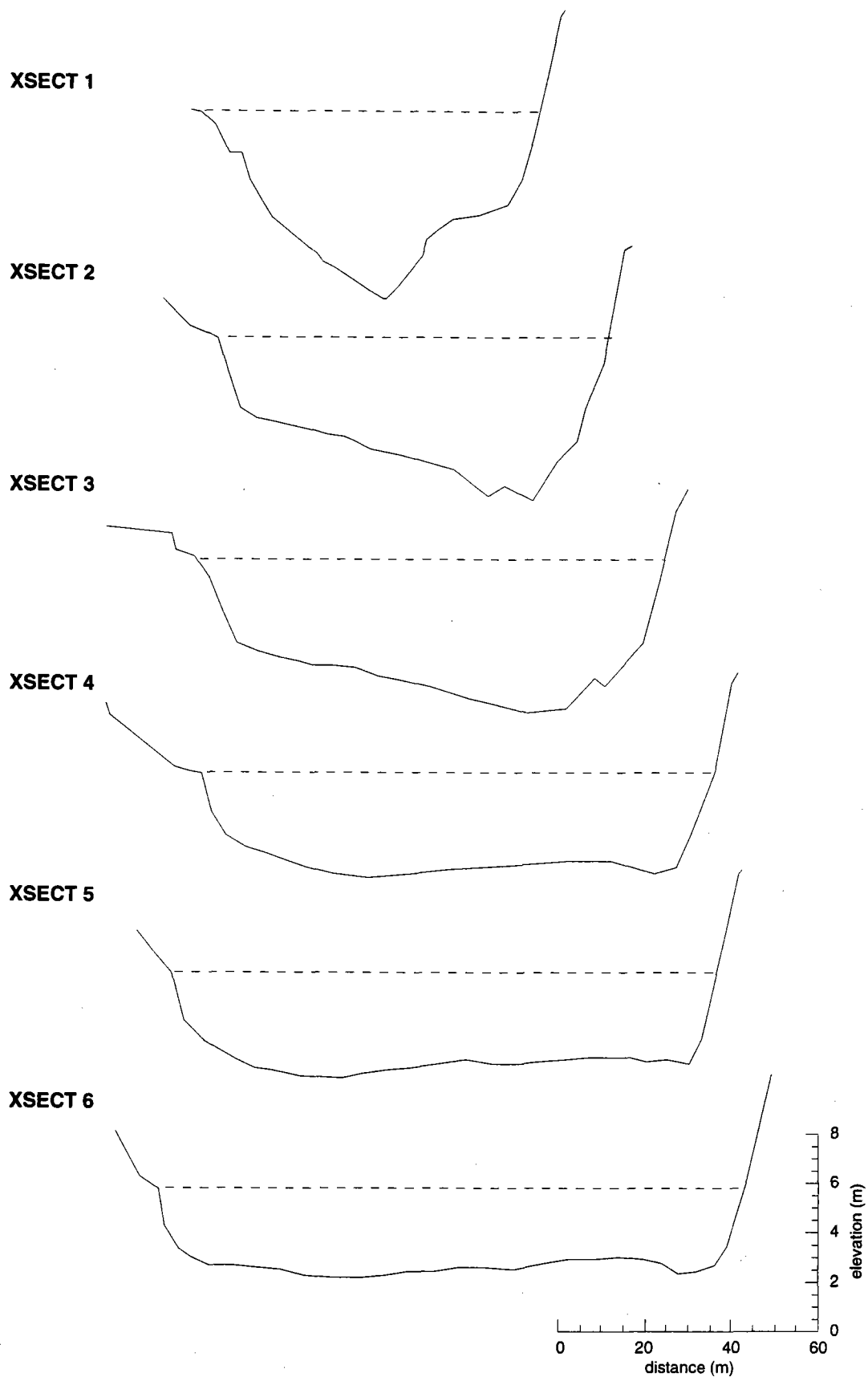
Figure 16. Main channel cross-sections of the Old Gauge site
