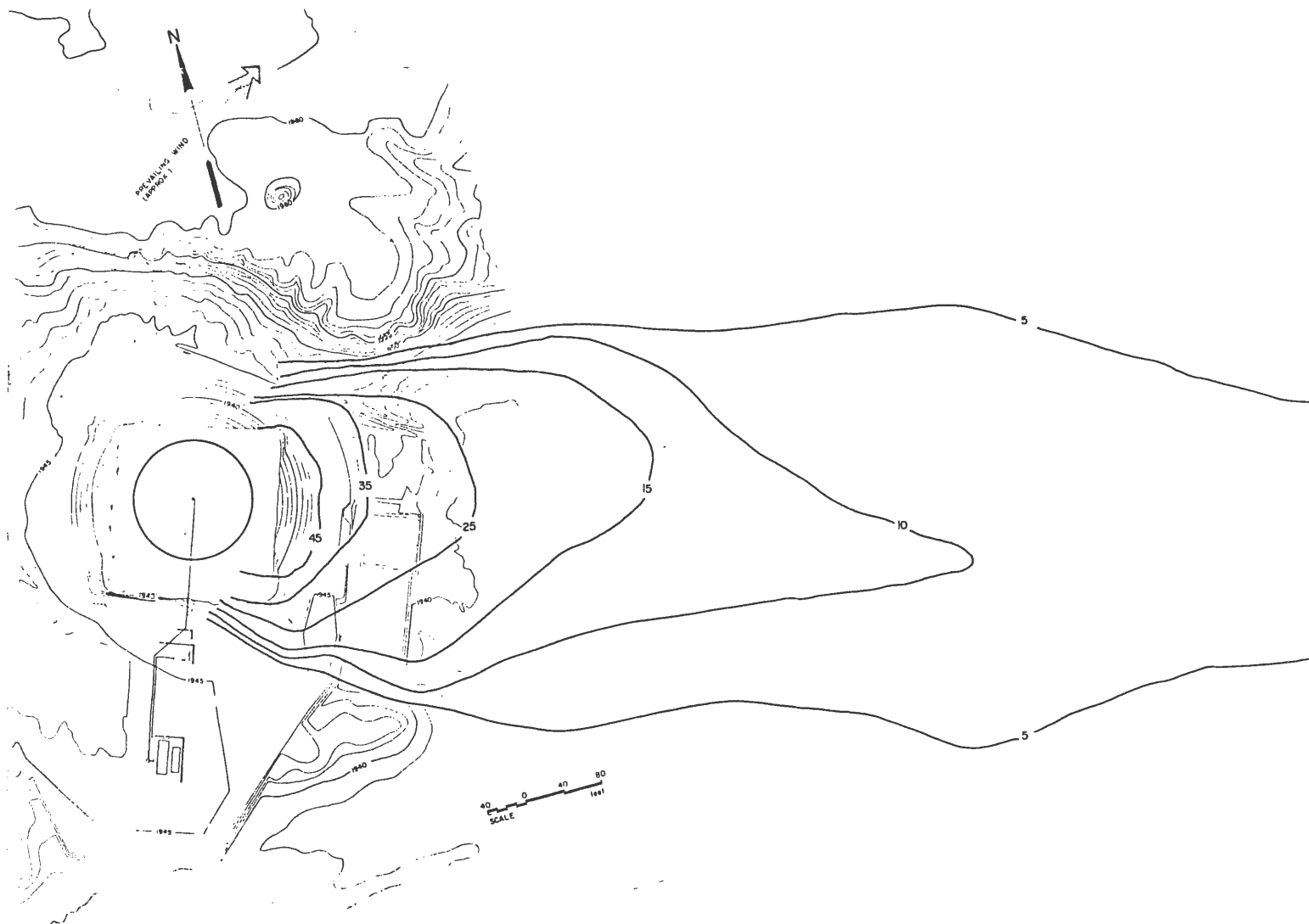
Figure 13-7. Ground Level Peak Concentration Contours (Run No. 7)
