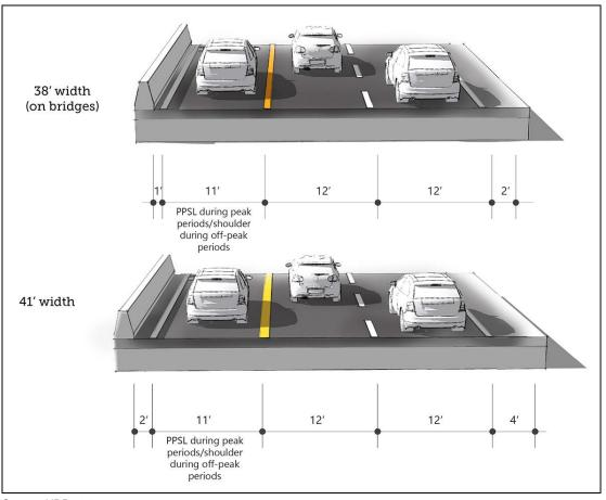
Figure 3. WB PPSL Proposed Action Typical Cross Sections
