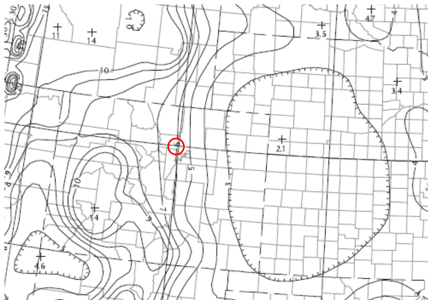
Figure B.6 - AASHTO Bridge Spec.: 3.10.2-1 Acceleration Coefficient for Conterminous United States (PGA) with Seven Percent Probability of Exceedance in 75 yr. (Approx. 1000-yr Return Period)
