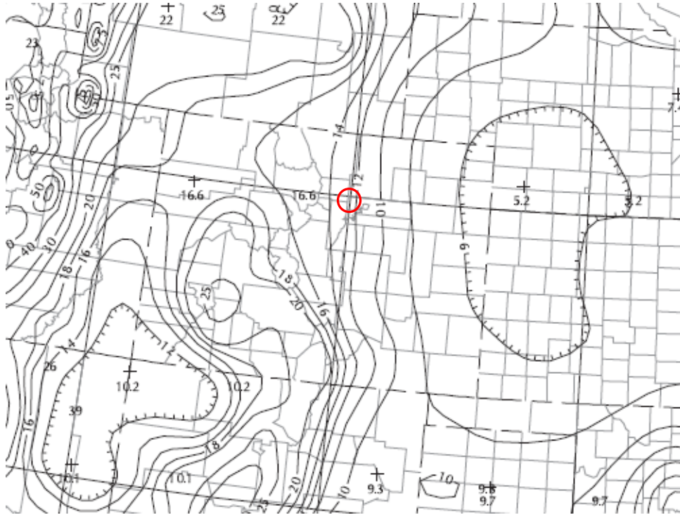
Figure B.7 – AASHTO Bridge Spec.: 3.10.2-2 Horizontal Response Spectral Acceleration Coefficient for the Conterminous United States at Period of 0.2 s ( S_s ) with Seven Percent Probability of Exceedance in 75 yr. (Approx. 100-yr. Return Period) and Five Percent Critical Damping
