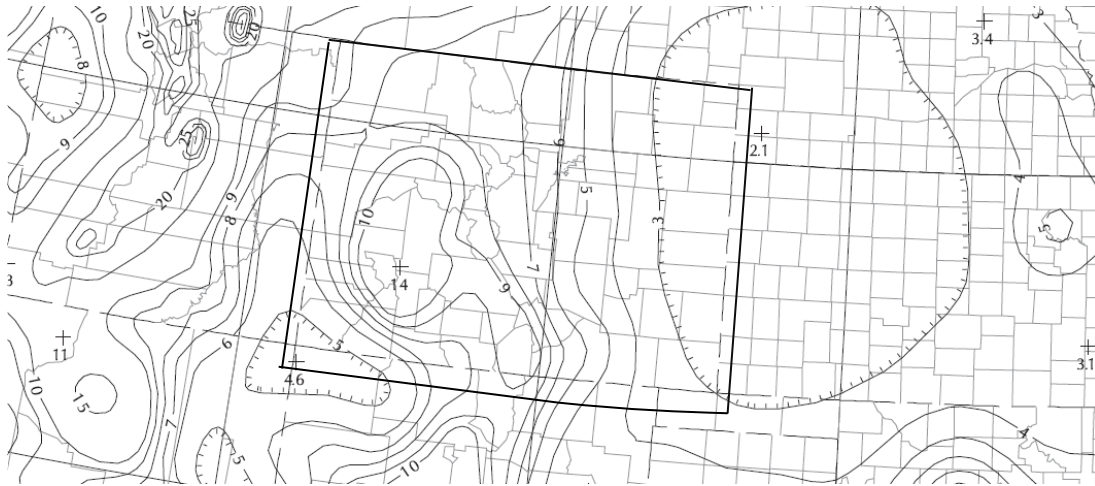
Figure 1.1 Seismic Hazard Maps for AASHTO Guide Specifications, Peak Ground Acceleration (PGA) (7% in 75-year) (2011)
