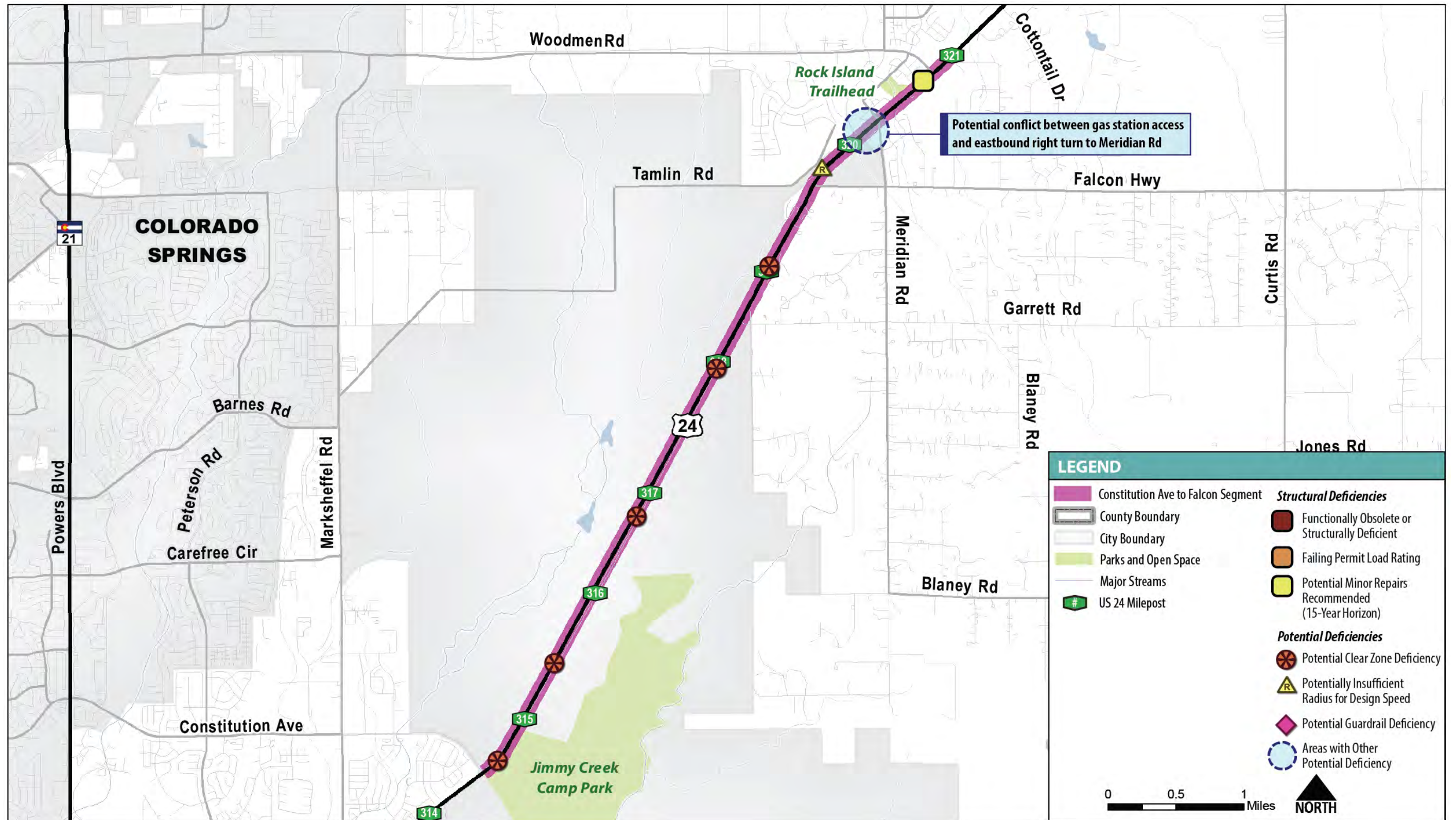
Figure 10: Roadway Conditions and Potential Deficiencies (Constitution Ave to Falcon)
