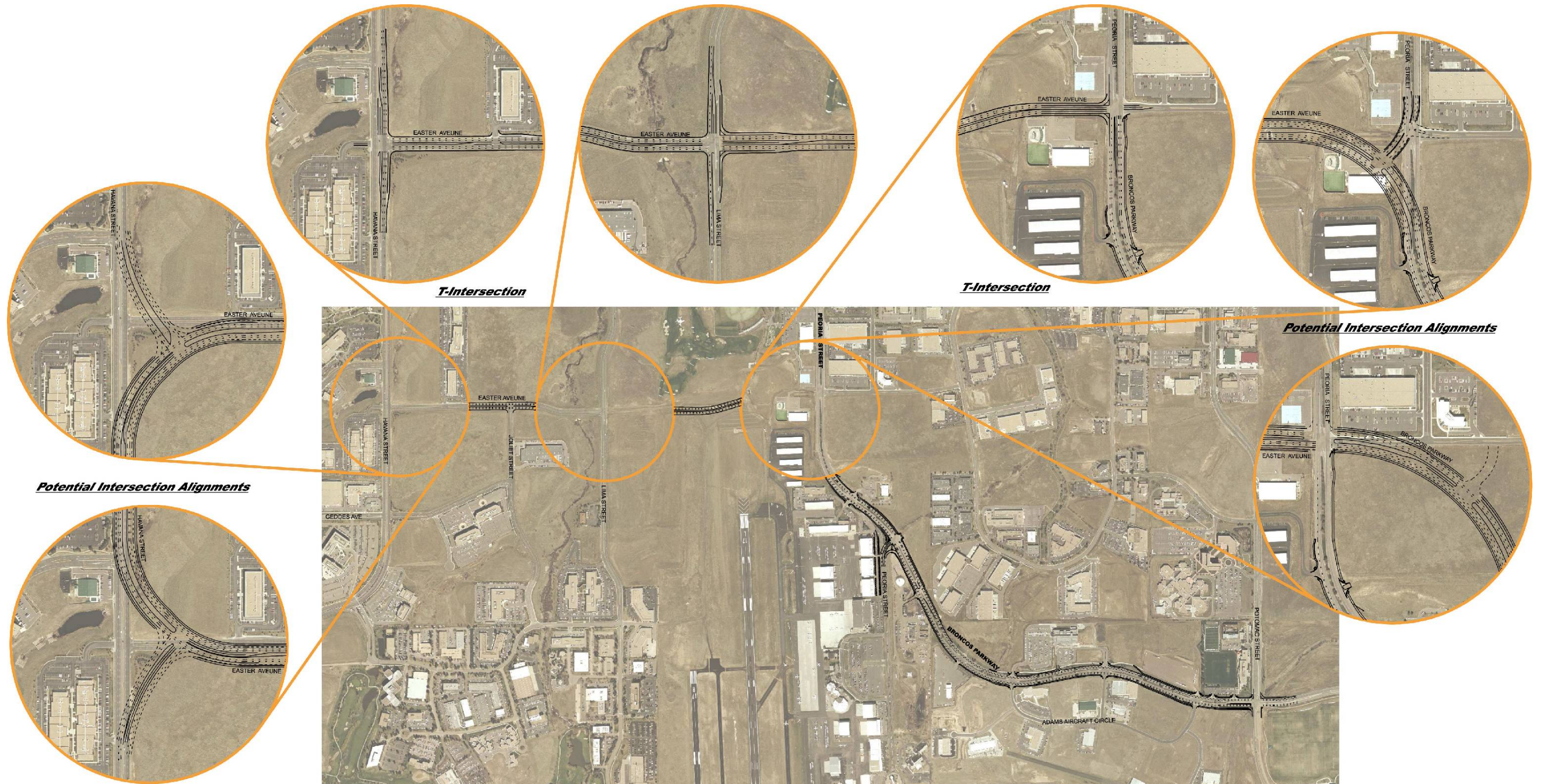
Figure A-3a. Havana/Easter/Peoria Intersection Alternatives and Planned Broncos Parkway Improvements, Easter to Potomac
