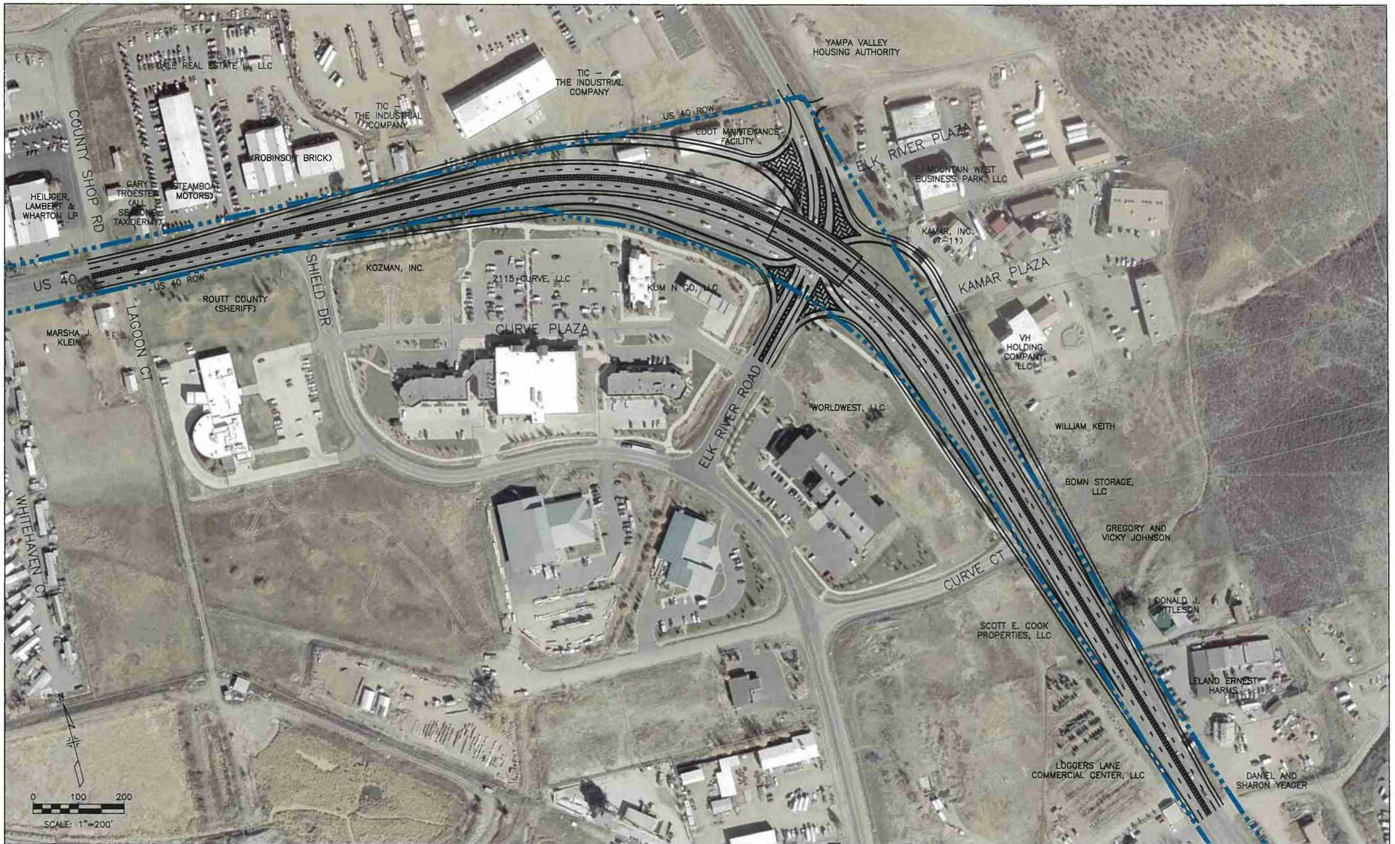
ELK RIVER ROAD SINGLE POINT URBAN INTERCHANGE ('SPUI') CONCEPT FIGURE 11 PAGE 49
