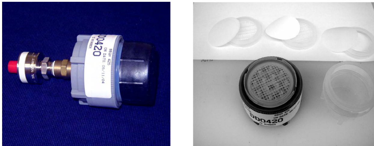
Figure 11.5. CASTNET filter pack ready for deployment (left) and a disassembled filter pack (right).
