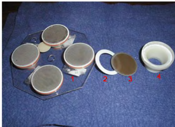
Figure 11.3. IMPROVE sampler filter cassette with additional screen and spacer for \text{NH}_3 collection. The sampler includes 1) cassette filter holder, 2) Teflon spacer, 3) Teflon-coated support grid, and 4) top of cartridge assembly.
