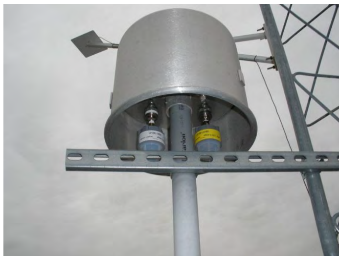
Figure 11.6. Regular (left) and modified (right) CASTNET filter packs in the sample holder.
