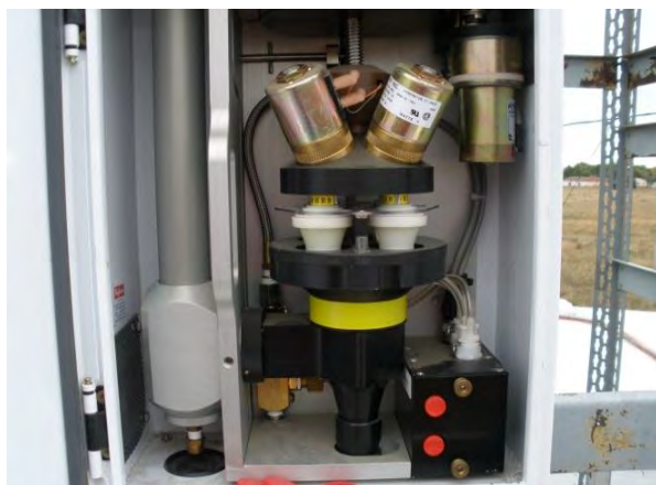
Figure 11.4. IMPROVE sampler channel B with sample cassette installed.
