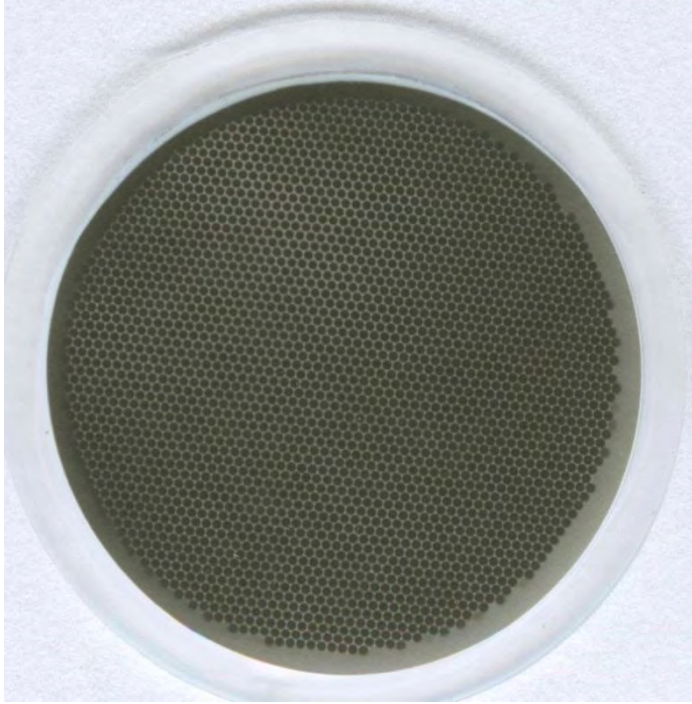
Figure 1.7. Filter sample collected using attached screen cassette.
