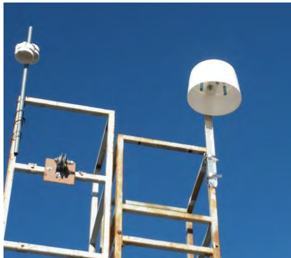
Figure 11.7. Passive samplers deployed in the field. The Ogawa sampler is on the left, and the Radiello sampler is on the right.
