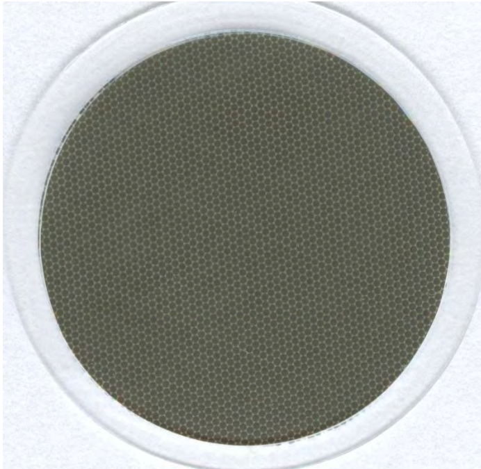
Figure 1.8. Filter sample collected using detached screen cassette.
