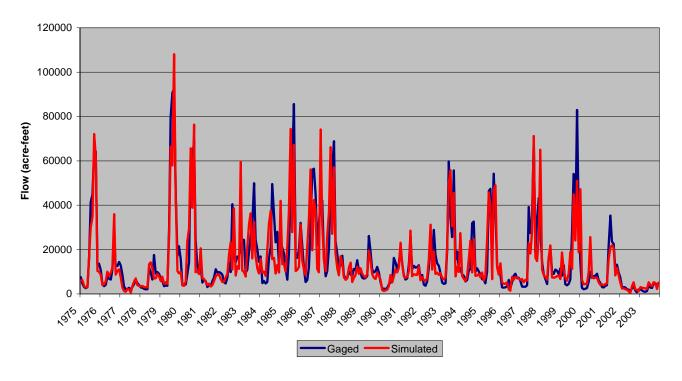
Figure D.4 Calculated Streamflow Simulation – Los Pinos River at La Boca
