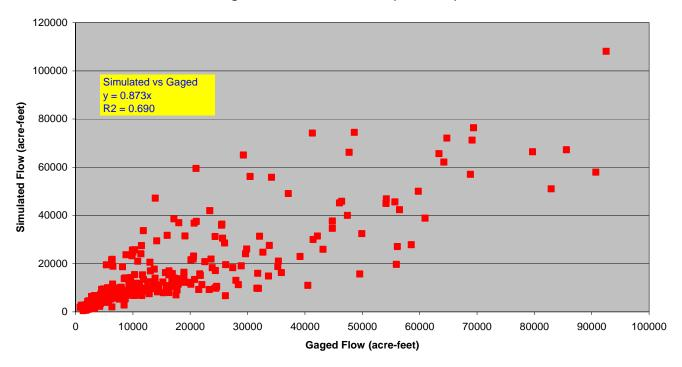
USGS Gage 09354500 - Los Pinos River at La Boca Gaged and Simulated Flows (1975-2003)
