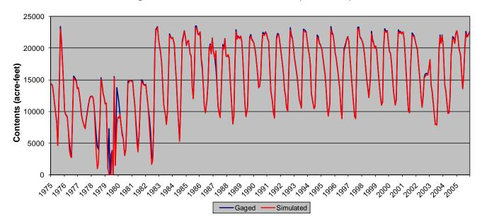
Figure 7.13 Reservoir Calibration – Cascade Reservoir
