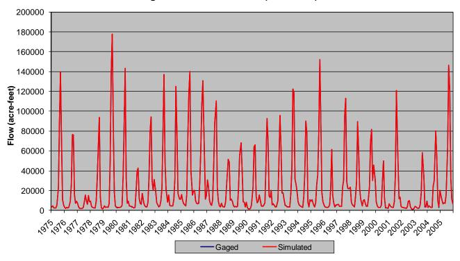
Figure 7.1 Streamflow Calibration – San Juan River at Pagosa Springs
