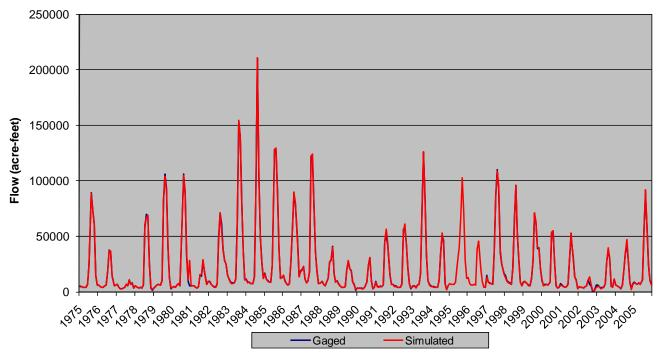
Figure 7.10 Streamflow Calibration – San Miguel River at Uravan
