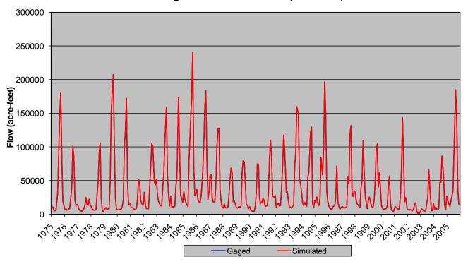
Figure 7.2 Streamflow Calibration – San Juan River near Carracus
