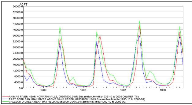
Figure 2 – Comparison of historical flows at gages 09357500, 09339900, and 09352900 for determination of which gage would best represent the mainstem of the San Juan River.
