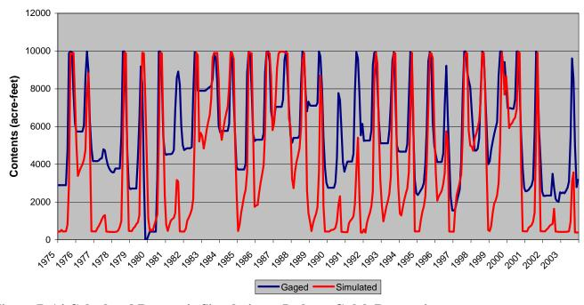
Figure D.14 Calculated Reservoir Simulation – Jackson Gulch Reservoir
