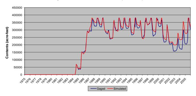
Figure 7.15 Reservoir Calibration – McPhee Reservoir
