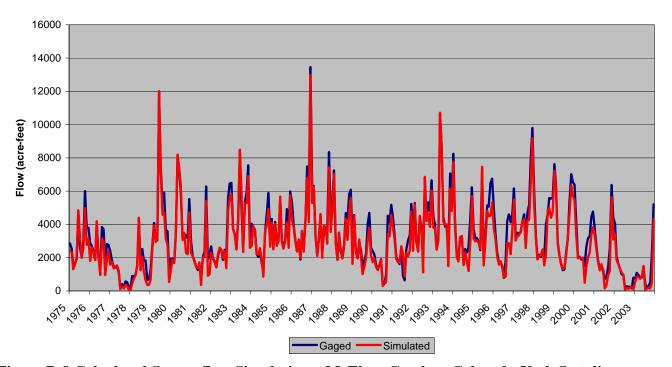
Figure D.8 Calculated Streamflow Simulation - McElmo Creek at Colorado-Utah Stateline
