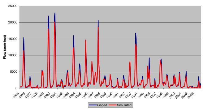
Figure D.6 Calculated Streamflow Simulation - La Plata River at Colorado-New Mexico Stateline
