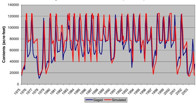
Figure D.11 Calculated Reservoir Simulation - Vallecito Reservoir
