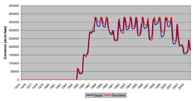
Figure D.15 Calculated Reservoir Simulation – McPhee Reservoir
