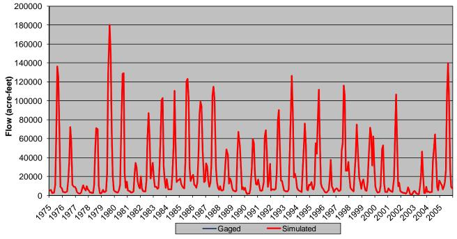
Figure 7.3 Streamflow Calibration - Piedra River near Arboles
