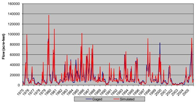
Figure 7.4 Streamflow Calibration - Los Pinos River at La Boca
