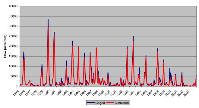
Figure D.7 Calculated Streamflow Simulation – Mancos River near Towaoc
