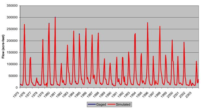
Figure D.5 Calculated Streamflow Simulation – Animas River at Durango
