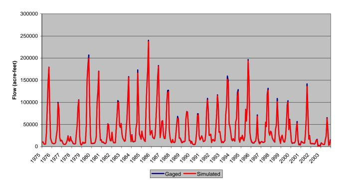
Figure D.2 Calculated Streamflow Simulation – San Juan River near Carracus
