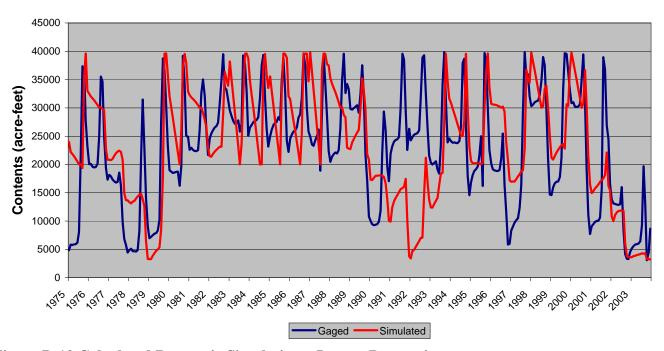
Figure D.12 Calculated Reservoir Simulation – Lemon Reservoir
