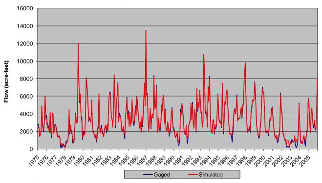
Figure 7.8 Streamflow Calibration - McElmo Creek at Colorado-Utah Stateline
