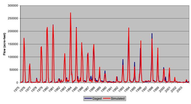
Figure D.9 Calculated Streamflow Simulation - Dolores River near Bedrock
