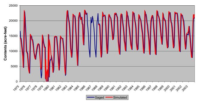
Figure D.13 Calculated Reservoir Simulation - Cascade Reservoir
