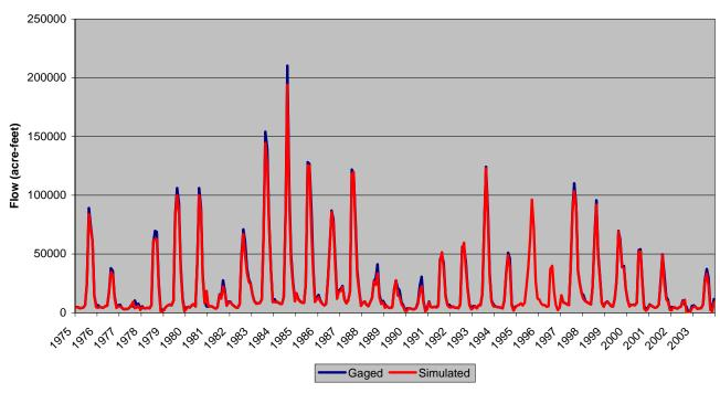
Figure D.10 Calculated Streamflow Simulation - San Miguel River at Uravan
