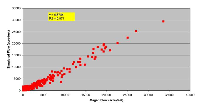
USGS Gage 09371000 - Mancos River near Towaoc Gaged and Simulated Flows (1975-2003)
