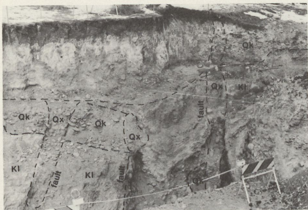
Figure 19. Photograph of east side of trench excavated across Golden Fault near Golden (Figure 1). Note faulted Kansan (?) deposits (Qk), especially the 18 ft (5.5 m) of offset along the far right fault. Zones of disoriented gravel clasts are labeled (Qx), and the Cretaceous Laramie Formation, (Kl) (generalized from Kirkham, 1977).
