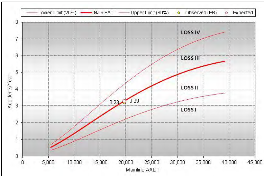
Figure 157 Four-Lane Divided Signalized Four-Leg Intersection Injury + Fatal Crashes per Year (22 nd Street) Minor AADT = 13,200
