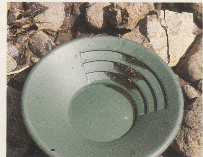
Figure 3e. Step 11, a green plastic pan with riffles showing dark, heavy mineral concentrate and spectacular, bright gold grains. (Photos by Jack Rathbone.)
