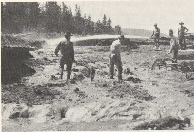
Figure 9. Miners ground sluicing with a monitor at Hahns Peak, Routt County. (Colorado University Historical Collections)
