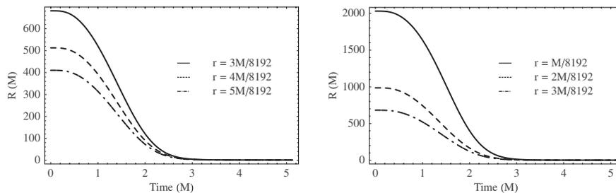
FIG. 9. Evolution of  $R$  for fixed  $r$  for the first  $5M$  of an extremely high-resolution simulation. Left panel: the evolution of the third, fourth, and fifth closest points to the puncture, at  $r = \{3, 4, 5\}M/8192$ , are shown. We do not expect the closest two points to be reliable, due to finite-difference errors across the puncture, although they show similar behavior, shown in the right panel.
