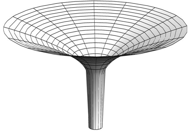
FIG. 2. Embedding diagram of a two-dimensional slice ( $t = \text{const}$ ,  $\theta = \pi/2$ ) of the maximal solution (17)–(20). The distance to the rotation axis is  $R$ . In contrast to Fig. 1 there is only one asymptotically flat end. The other end is an infinitely long cylinder with radius  $R_0 = 3M/2$ .
