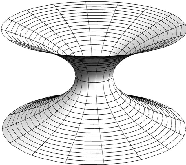
FIG. 1. Embedding diagram of a two-dimensional slice ( $T = \text{const}$ ,  $\theta = \pi/2$ ) of the extended Schwarzschild solution. The distance to the rotation axis is  $R$ . A wormhole with a throat at  $R = 2M$  connects two asymptotically flat ends.
