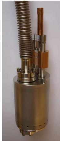
**Figure A.1.:** Cryogenic vacuum valve, shown in a assembly that was used to leak test the valve in the vacuum mode. The holes seen at the bottom of the valve body are used to vent the gases form screw threads of the indium seal.
