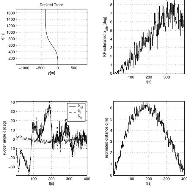
Fig. 5. Closed-loop simulation results for the KF-estimation of a constant disturbance  $\Delta\alpha_w = 7^\circ$  with  $\alpha_w = \alpha_{GL} + \Delta\alpha_w$ .
