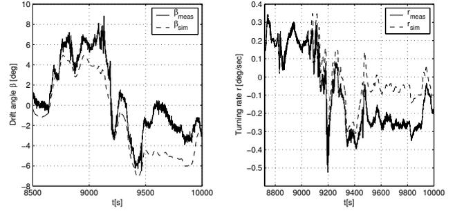
Fig. 4. Measured and simulated drift angle  $\beta$  and turning rate  $r$ .
