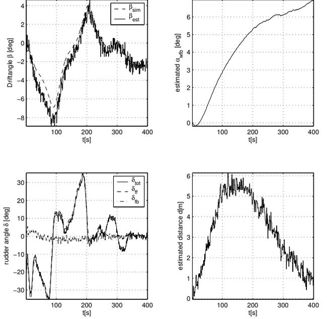
Fig. 6. Closed-loop simulation results for the estimation of a constant disturbance  $\Delta\alpha_w = 7^\circ$  with  $\alpha_w = \alpha_{GL} + \Delta\alpha_w$ .
