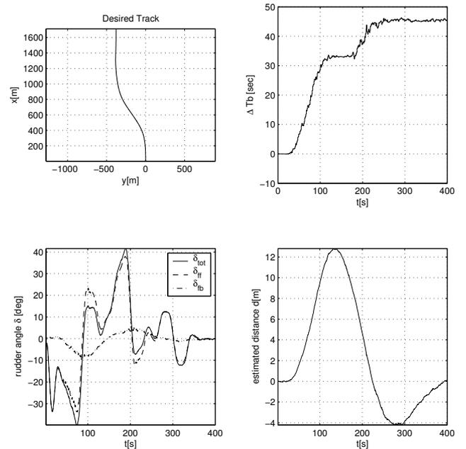
Fig. 9. Closed-loop simulation results for  $T_B^N = 100\text{sec}$  and estimation of  $\Delta T_B^N$ .
