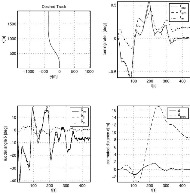
Fig. 10. Closed-loop simulation results for  $\delta_{off} = 10$  and  $T_r^N = 44$ ,  $d_{prev}$ ..distance without estimation of  $r_w$ .
