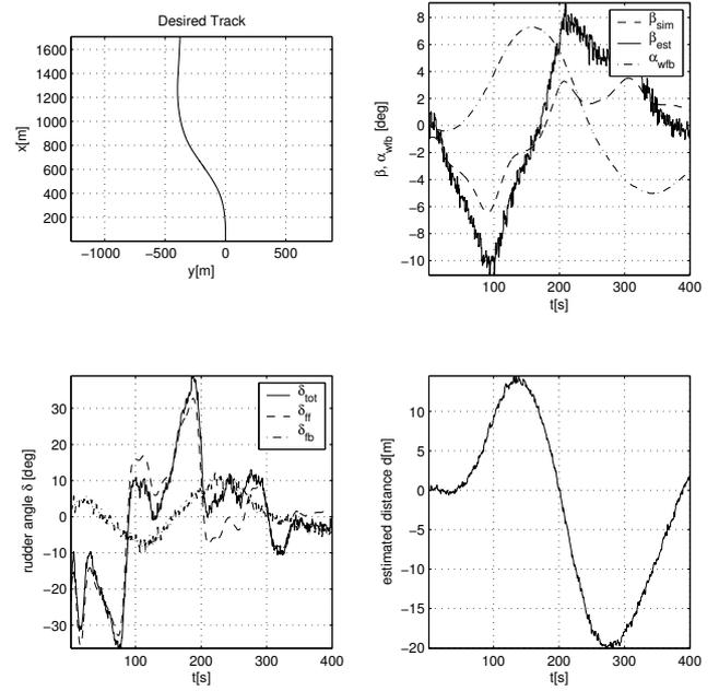
Fig. 8. Closed-loop simulation results for  $T_B^N = 100\text{sec}$ .
