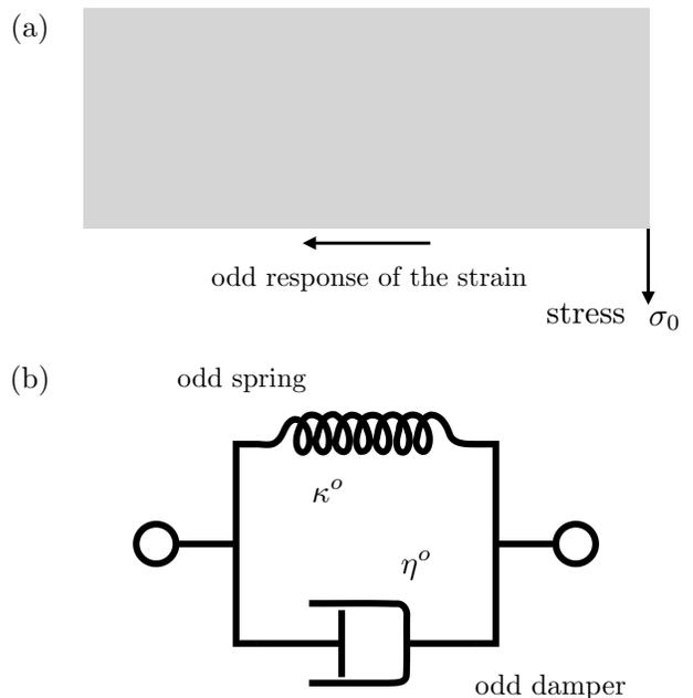
FIG. 1: (a) A sketch of the odd Kelvin-Voigt model. Upon application of a constant stress the resulting deformation will be perpendicular to the stress direction. The decay of the deformation will be captured by odd transport coefficients. (b) Depiction of the odd response in odd Kelvin-Voigt materials. It is modelled by a transverse spring and a damper connected in parallel.
