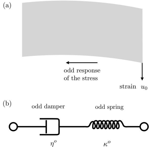
FIG. 2: (a) A cartoon of the odd Maxwell model. A finite deformation will result in a transverse stress. Its relaxation will be captured by odd transport coefficients. (b) Depiction of the odd response in odd Maxwell materials. It is modelled by a spring and a damper connected in series. We emphasize that this collective representation *does not* imply that odd Maxwell fluids can be constructed out of springs and dampers.
