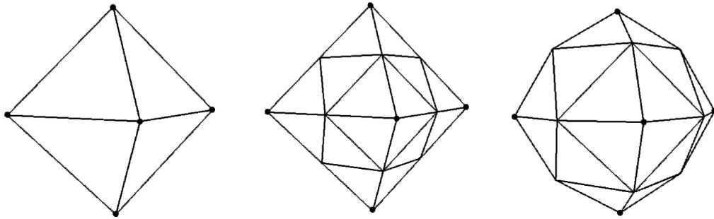
Fig. 2. Subdivision of an octahedron. Each face of the mesh is split into four triangles and the resulting mesh is smoothed by shifting the vertices. Even vertices in the refined mesh are marked by solid bullets.
