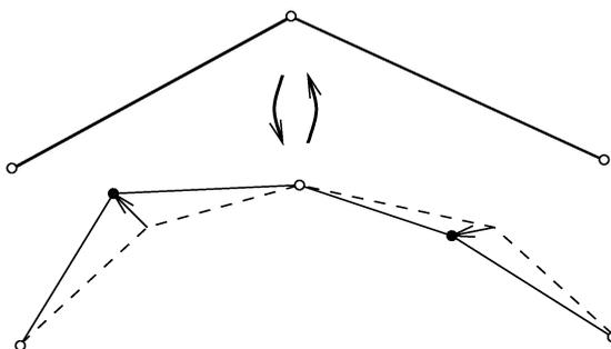
Fig. 7. The solid line below represents the original fine mesh  $\mathcal{M}^{k+1}$ , the solid line above the coarsified mesh  $\mathcal{M}^k$ . Applying the subdivision operator  $S$  to  $\mathcal{M}^k$  yields the dashed line which interpolates  $\mathcal{M}^{k+1}$  at the even vertices. By eventually adding the detail vectors to the odd vertices, the original mesh can be reconstructed.
