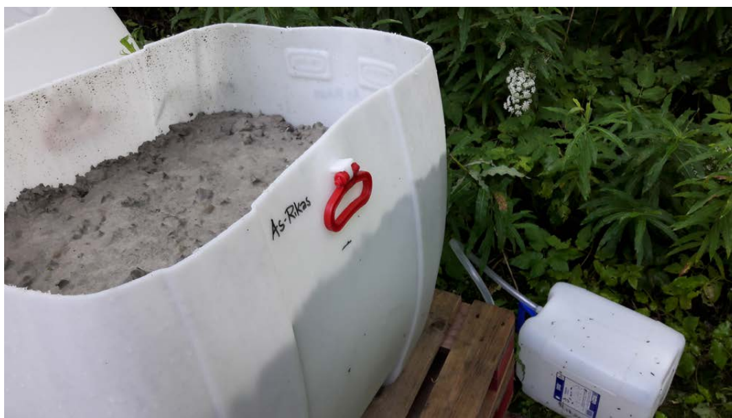
Fig. 2. Plastic lysimeter filled with As-rich tailings and drainage water canister in Kuopio in summer 2016. Photo by A. Tornivaara, GTK
