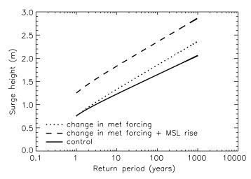
**Figure 11.14:** Frequency of extreme water level, expressed as return period, from a storm surge model for present day conditions (control) and the projected climate around 2100 for Immingham on the east coast of England, showing changes resulting from mean sea level rise and changes in meteorological forcing. The water level is relative to the sum of present day mean sea level and the tide at the time of the surge. (From Lowe *et al.*, 2001.)
