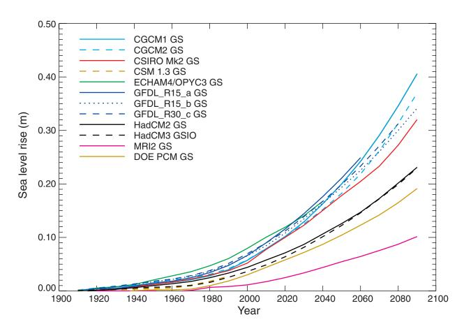
**Figure 11.1:** Global average sea level changes from thermal expansion simulated in AOGCM experiments with historical concentrations of greenhouse gases in the 20th century, then following the IS92a scenario for the 21st century, including the direct effect of sulphate aerosols. See Tables 8.1 and 9.1 for further details of models and experiments.
