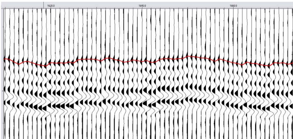
Figure 7: Typical direct arrival picked in order to analyse the “jitter” variations in the firing trigger and correct for them.
