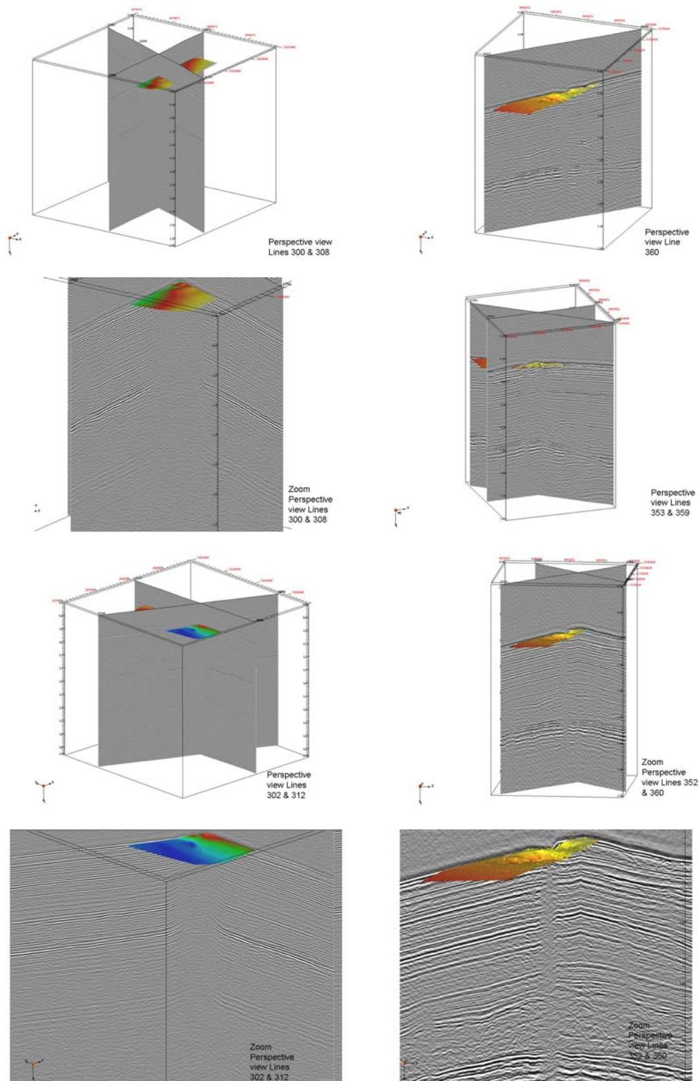
Figure 12: Screen shots from Kingdom showing perspective lines through the CN03 (left column) and G11 (right column) pockmarks illustrating the generally good agreement between intersecting lines and the bathymetry. Generally it was found that the CMP locations were better constrained at the CN03 pockmark when compared to the G11 pockmark.
