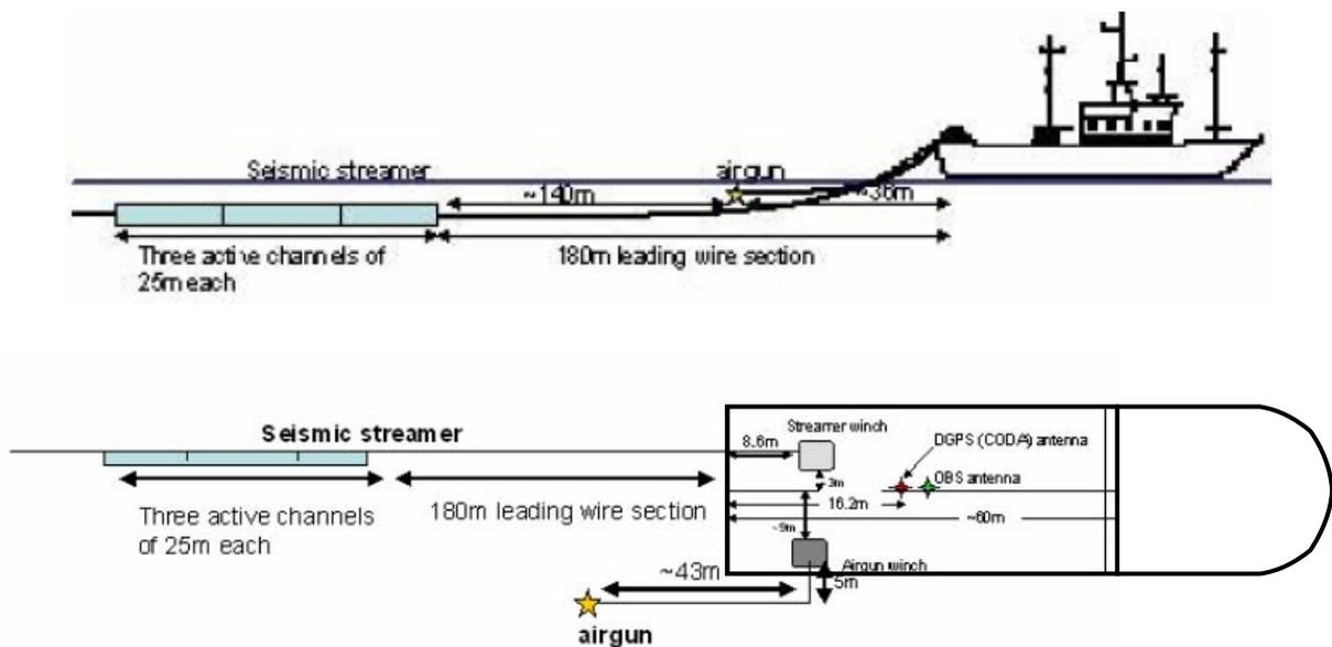
Figure 4: Schematic illustrating streamer airgun configuration.
