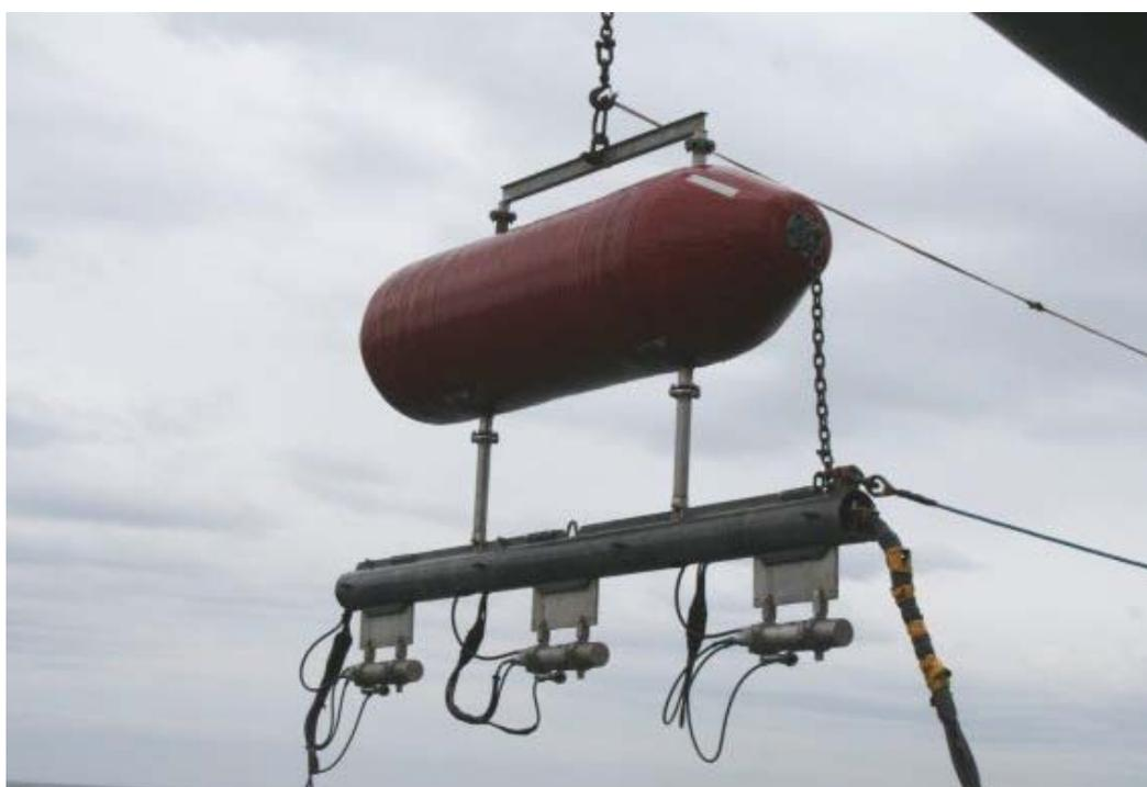
Figure 5: Mini GI-gun setup used as the seismic source for the streamer lines.
