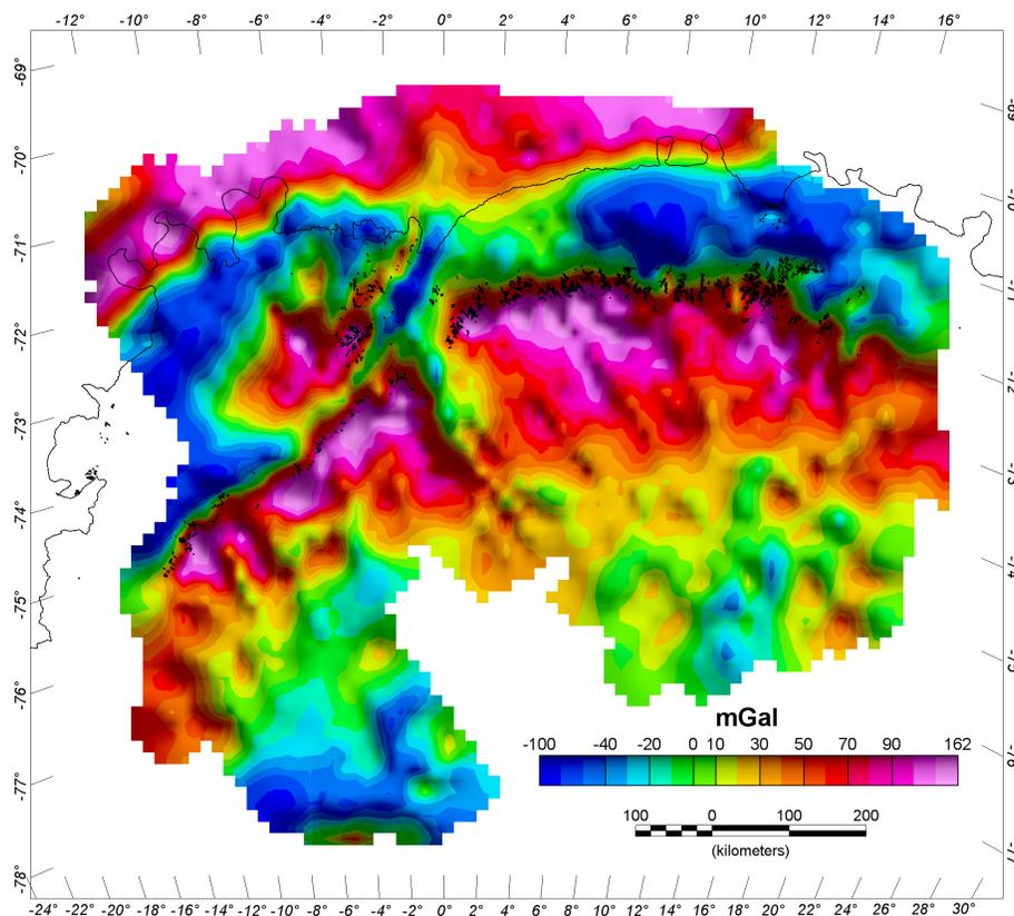
**Figure 2.** Compilation of preliminary results of the Free-Air Anomaly Map, gridded cell size is 15km.
