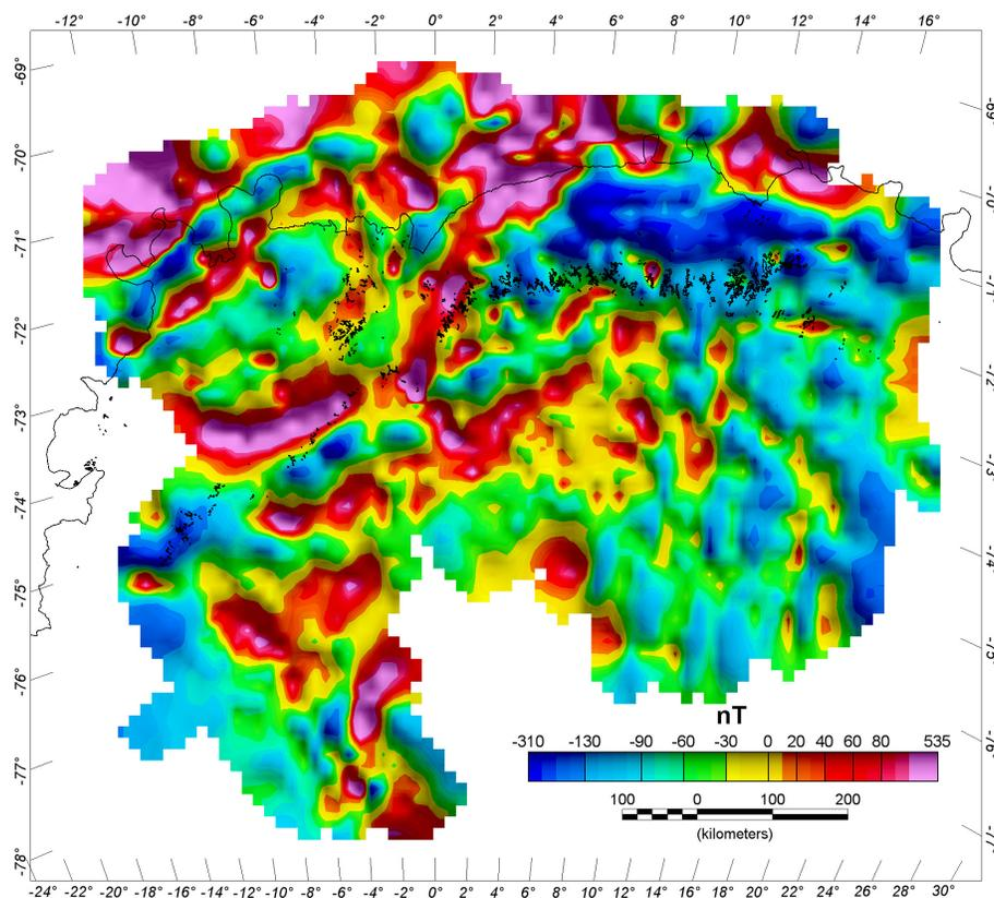
**Figure 1.** Compilation of preliminary results of the Magnetic Anomaly Map, gridding cell size is 15km.
