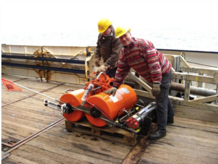
*Fig. 4.3: Ocean-bottom seismometer (OBS) after recovery from the sea-floor*
