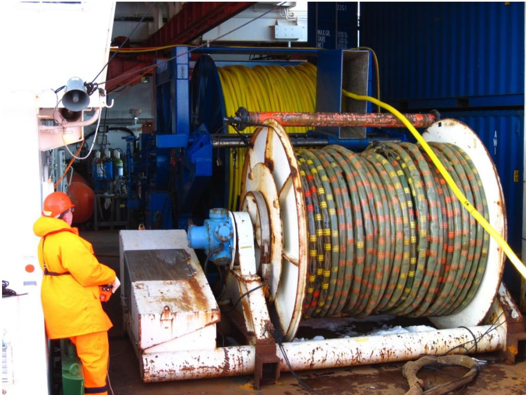
*Fig. 4.1: Winches with the 600 m streamer (in front) and the 3,000 m streamer (in the back) on the working deck.*
