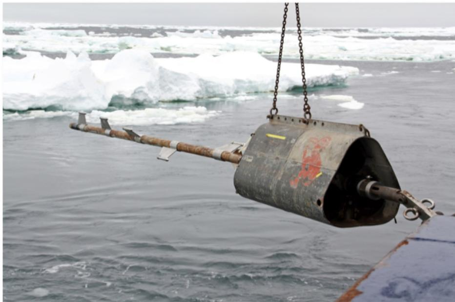
*Fig. 4.9: Temperature gradient probe equipped with five temperature loggers on the lance and one on the head for bottom water reference temperature.*
