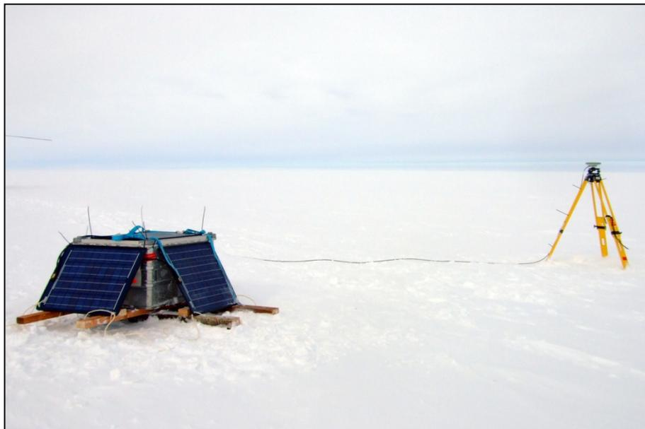
*Fig. 8.4: Set-up of the GPS equipment at site GET1 on the Getz Ice Shelf*
