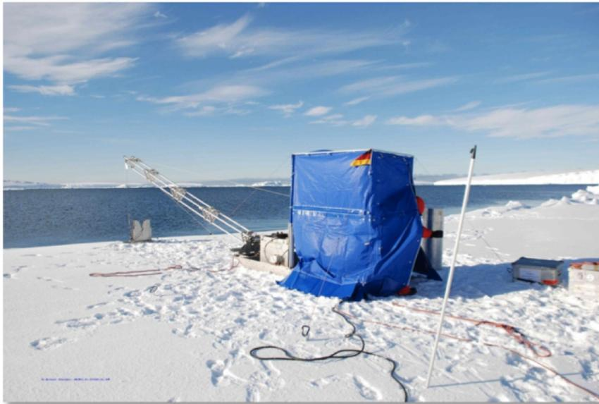
*Fig. 6.6: Fully rigged up measuring system on site 26-01. It consists of a tent, the winch, and a maneuverable mast. Online data acquisition is done via the deck unit on a laptop in the tent. The mast allows the CTD to hang aside the floe without touching the ice. For transportation the mast can be disassembled into 4 pieces of 1m length. The generator sledge is not seen.*
