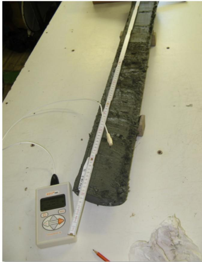
*Fig. 4.10: Thermal conductivity measurement on split cores using the KD2 Pro instrument*
