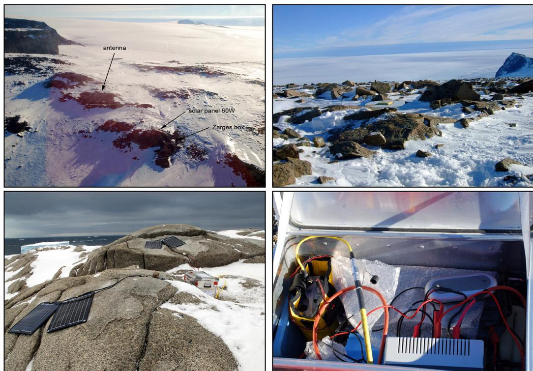
*Fig. 8.2: Installation of the GPS equipment at the sites MANT (upper left), BEAR (upper right) and PIG2 (lower left). The lower-right photograph shows the typical set-up of receiver, batteries and auxiliary devices within the Zarges aluminium box.*
