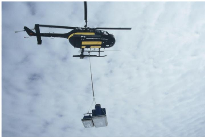
*Fig. 6.4: Portable CTD system carried by a helicopter. For protection all components are covered by a canvas.*
