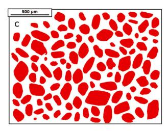
**Fig. 2.** (a) Photographic image of ikaite crystals in slush. Owing to the overlap of ikaite crystals (a), ImageJ software could not extract each crystal. Therefore, each crystal was outlined by visually drawing a red line around its perimeter (b) and moved to eliminate the overlap between crystals (c). Each crystal was then colored red and extracted according to its brightness using ImageJ. Note that crystals touching the edge of the image were excluded from the analysis.
