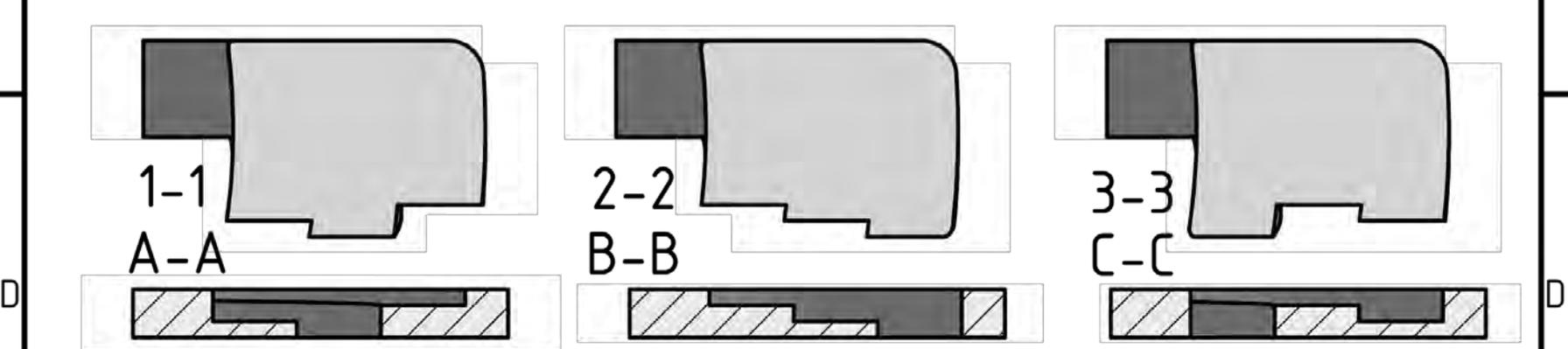
The design of the cutters is based on the idea of Victor Zagorodnov by having cut 1/3 with a 1/3 wide cutter, the next 1/3 is cut by a cutter which is 2/3 wide and the last 1/3 is cut by a full cutter. The drawback of Victor's head in my opinion is that the pitch is still set by screws, in our case shoes. Of course Victor will argue that there is alcohol, but in our hole we try to avoid alcohol. The design guideline for the new cutters was to set the pitch
