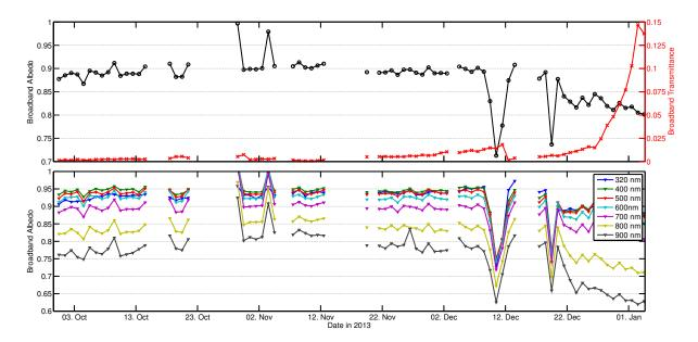
Figure 20: Broadband albedo and transmittance (top) and albedo at selected wavelengths (bottom).
