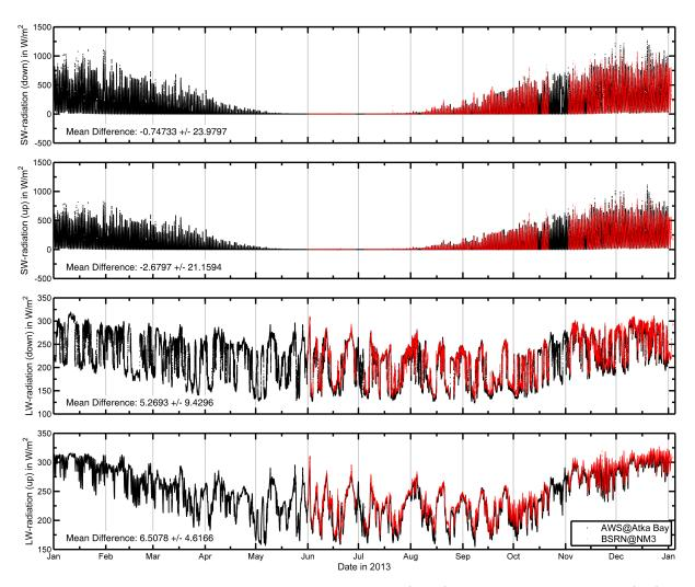
**Figure 13:** Radiation measurements at Neumayer III (black) and on Atka Bay fast ice (red) in 2013. a) Downward short-wavelength radiation (SWD); b) upward short-wavelength radiation (SWU); b) downward long-wavelength radiation (lwd); b) upward long-wavelength radiation (LWU);
