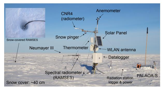
Figure 11: Setup of autonomous measurements at ATKA03 on 18 September 2013.
