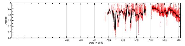
Figure 14: Albedo at ATKA03, calculated from down- and upward long-wave radiation. The daily average is shown in black.
