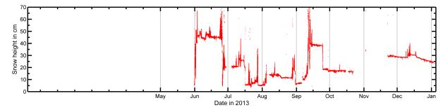
Figure 16: Snow depth at ATKA03, calculated from ultrasonic snow pinger (temperature corrected).
