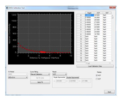
Figure 7: EM31 calibration on 16 December 2013. The red crosses are the data points from the calibration, the squares represent the 1-D exponential model best fitting to the data. The calibration coefficients for all data presented in this report are found in the lower box.
