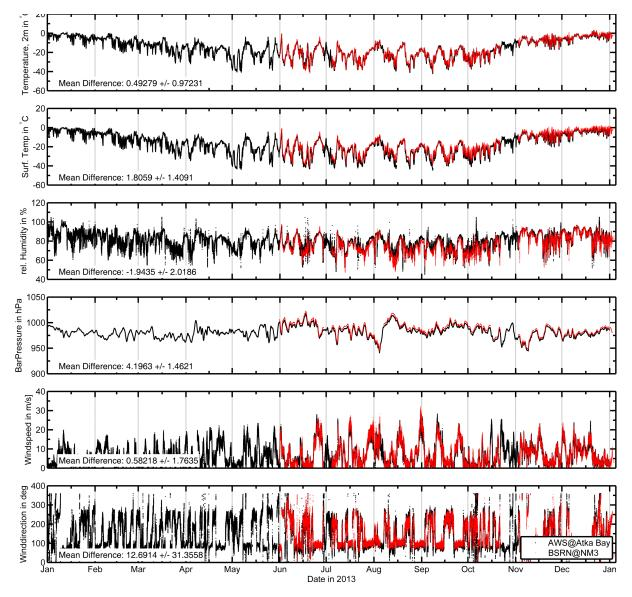
**Figure 12:** Meteorological measurements at Neumayer III (black) and on Atka Bay fast ice (red) in 2013. a) 2 m air temperature; b) surface temperature calculated from upward long-wavelength radiation; c) relative humidity; d) barometric pressure; e) windspeed; f) wind direction (from North).
