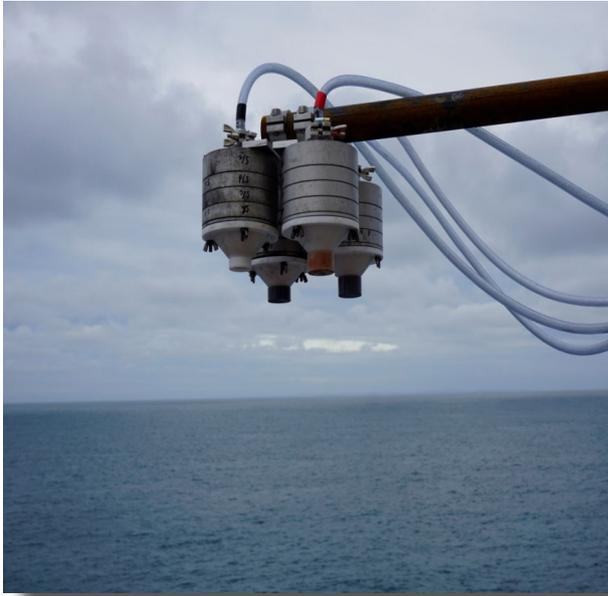
Fig. 3.7.1: Four filter pack systems collecting samples of NH<sub>3</sub> and NH<sub>4</sub><sup>+</sup>
