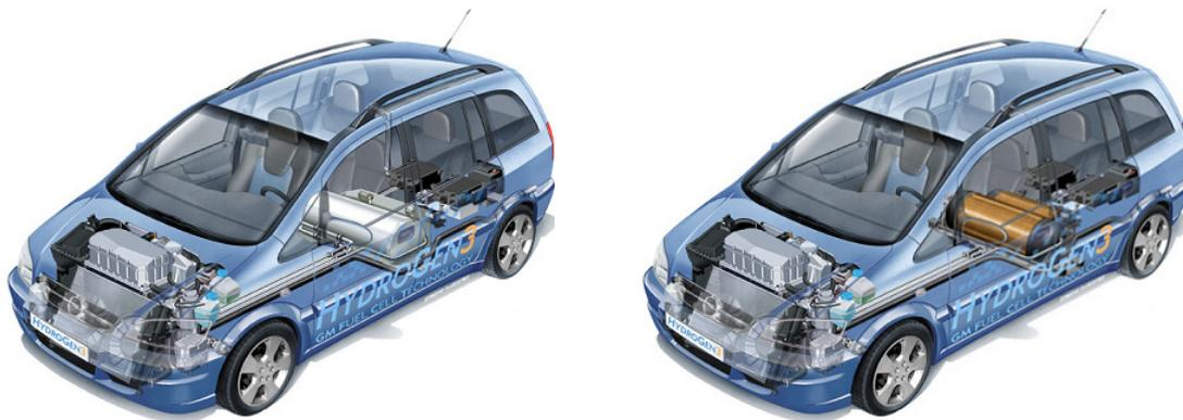
**Figure 1:** Opel's prototype hydrogen cars HydroGen3. Left: vehicle with liquid hydrogen tank, right: vehicle with compressed hydrogen gas tank (700 bar)
