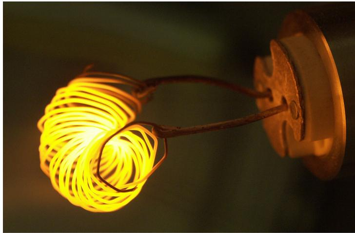
**Figure 5.3:** Photograph of the heating wire with the more efficient winding, as mentioned in section 5.3.2.
