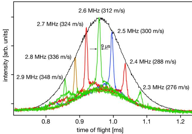
FIG. 3 (color online). Arrival time distributions of metastable CO molecules, for seven different frequencies  $\omega/2\pi$ , corresponding to velocities of the traveling potential wells ranging from 276 to 348 m/s. The enveloping curve is the arrival time distribution of the molecules in free flight, scaled down for this comparison.
