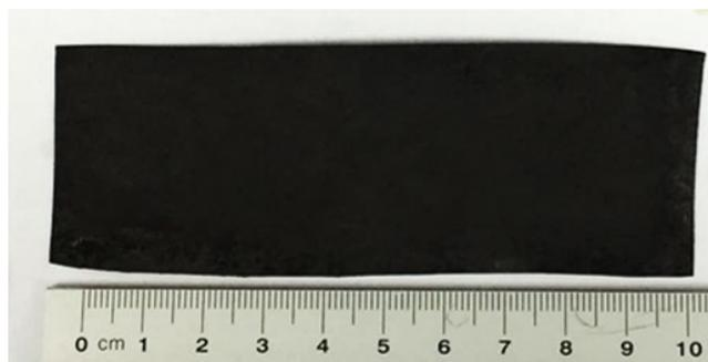
**Supplementary Figure 29 | A large piece of HNDCM-100,000-1000/Co catalyst with a size of 10.5 x 3.5 cm<sup>2</sup> and thickness of ~70 μm.** This membrane is the largest one that we can prepare using our carbonization oven at 1000 °C in our lab. The membrane size can be even larger if larger carbonization ovens are available.
