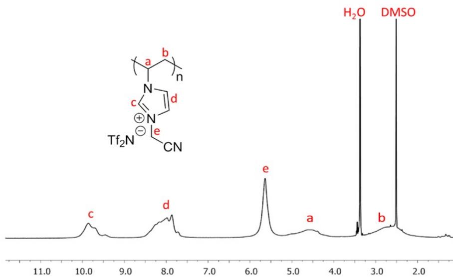
Supplementary Figure 1 |  $^1\text{H-NMR}$  spectra of PCMVImTf<sub>2</sub>N in DMSO-*d*<sub>6</sub>.
