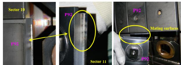
Figure 3 Damages on the P92 tiles in AUG: on the left hand side are shown the arc damages and on the right hand side the mating contact surface between tiles.
