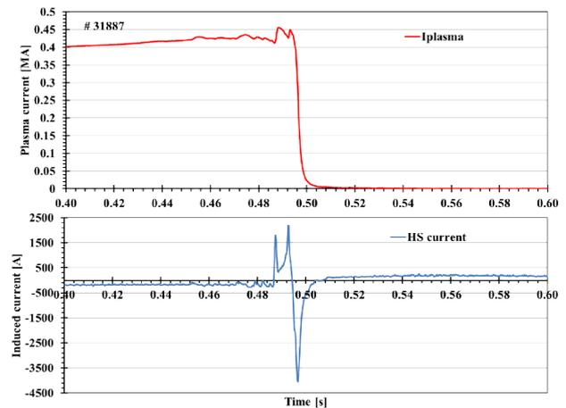
Figure 7 Induced current in the HS measured by the Rogowski coil for the shot # 31887: in correspondence of the plasma current disruption the current in the frame support increases.
