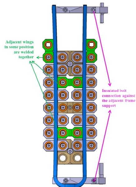
Figure 9 Modifications to the HS supporting structure are highlighted: in green welding between adjacent wings and in pink the electrical insulation between adjacent HS.
