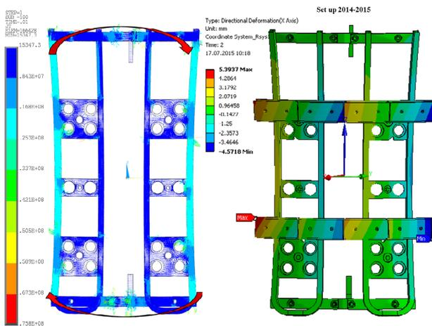
Figure 5 On the left: current density path through the HS structure for a uniform variation of radial field. On the right: corresponding displacement [mm] caused by 35 kN radial forces.
