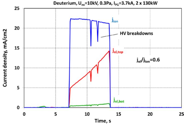
FIGURE 4. Extracted current densities the ions and the electrons in a 6.4 s pulse in deuterium
