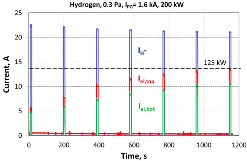
FIGURE 3. 1160s pulse in hydrogen with the 125 kW power limit for the co-extracted electrons on the extraction grid halves
