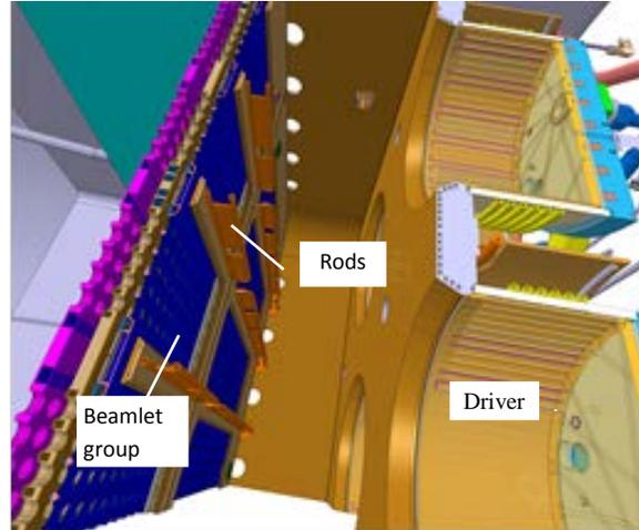
**FIGURE 5.** Cut of the ELISE source with three rows of rods between the beamlet groups
