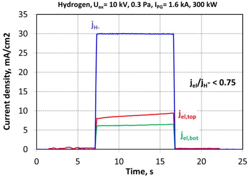
FIGURE 2. Extracted current densities of the ions and the electrons in a 10s pulse in hydrogen
