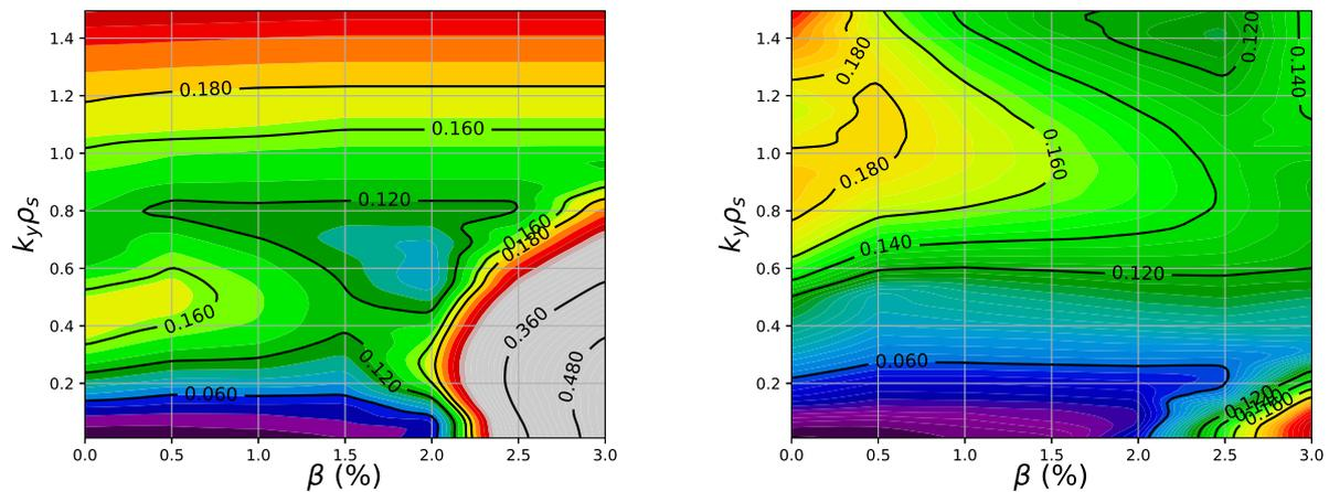
Figure 3: Instabilities growth rates as a function of  $\beta$  and  $k_y \rho_s$  (colorcoded), when pressure gradients are not (!) consistent with the plasma equilibrium. Left: simulations for standard tokamak case. Right: W7-X standard configuration (KJM, "bean" tube).
