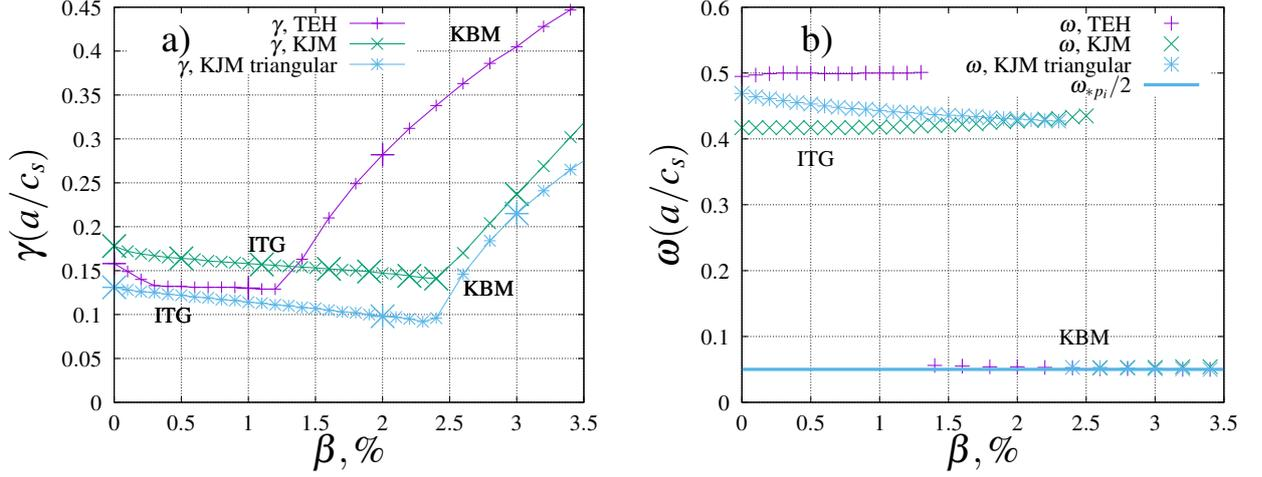
Figure 1: Fastest growing mode dependence on  $\beta$  for the with  $a/L_{Ti,e} = 2$  and  $k_y \rho_s$  in the range from 0.05 to 0.8, in two different W7-X configurations (KJM and TEH) and two simulation tubes (centred around the outboard midplane of the "bean" and "triangular" plane). (a): growth rate of the instabilities. (b): real frequency of the corresponding modes. Large dots specify where the magnetic equilibrium was varied.
