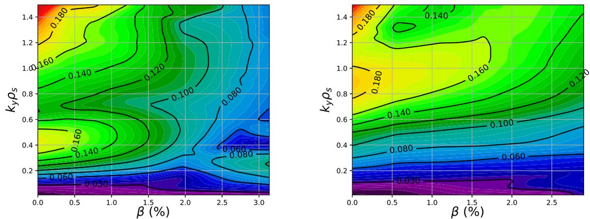
Figure 2: Instabilities growth rates as a function of  $\beta$  and  $k_y\rho_s$  (colorcoded), when pressure gradients are consistent with the plasma equilibrium. Left: simulations for standard tokamak case. Right: W7-X standard configuration (KJM, "bean" tube).
