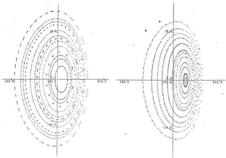
Fig. 3: Magnetic surfaces of Wendelstein VII A at finite  $\beta$ . left:  $\beta(0) = 0.5\%$  right:  $\beta(0) = 1.5\%$
