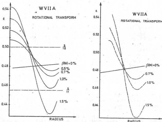
Fig. 2b (right):  $\epsilon$ -profile of W VII-A as a function of plasma pressure. 2a(left):  $\epsilon$ -profile W VII-A from AJW-code.
