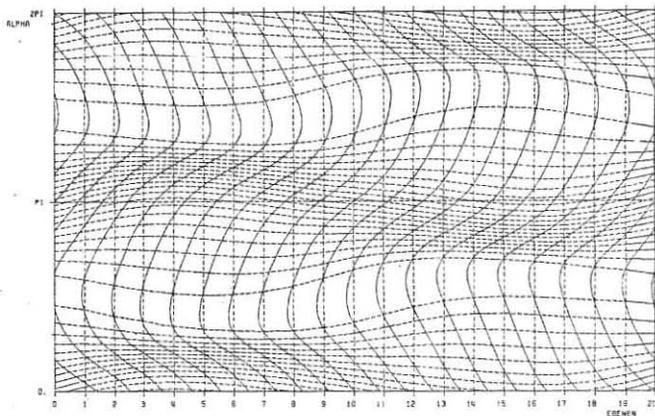
Fig. 1: Plasma currents on a magnetic surface of W VII-A (solid lines).
