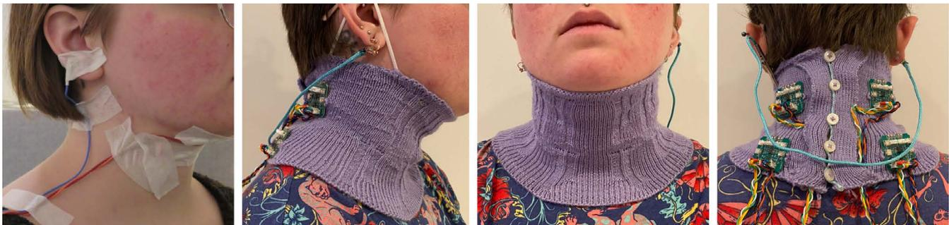
**Figure 11:** Reed wearing the completed knit collar, showing the knit's form on the neck compared to the original EMG setup.
