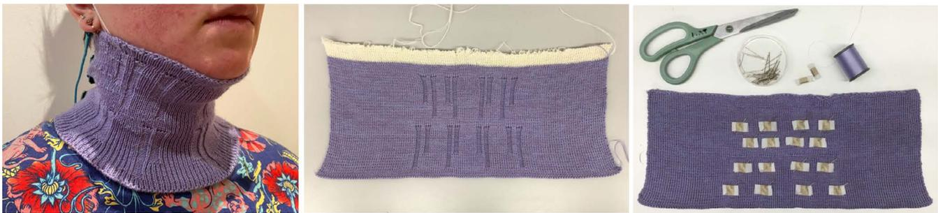
**Figure 1:** The *Singing Knit*, worn by Reed (left). Alternating ribbing on the outside of the collar highlights the position of the muscles and electrode placements (middle). Fabric electrodes made from zebra jersey are stitched by hand into the correct locations (right).
