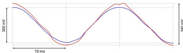
**Figure 12:** The vectorized signals from rigid electrode setup (red) and the fabric electrodes (blue) stitched into the collar. The signals measured are from the activation of the omohyoid during the singing exercise, as captured by the oscilloscope.
