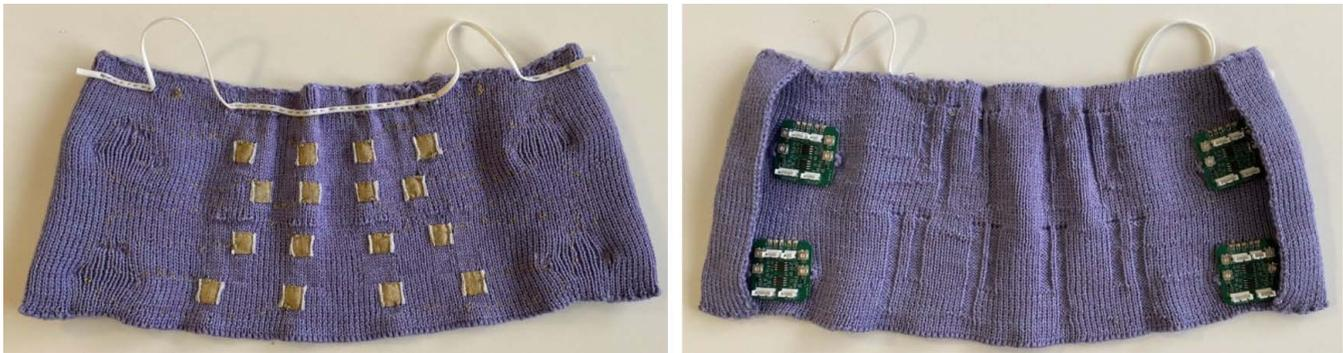
**Figure 10:** Amendments made to the collar: additional elastic is added to the inside of the collar to hold it up around the chin and provide support with straps around the ears (left). The excess fabric is folded over on the back to ensure a tight fit (right); these ends will be joined once the collar is on the wearer.
