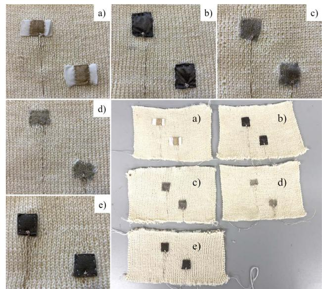
**Figure 6:** Swatches with stitched, soft fabric electrode probes for comparing materials. In order: a) silver-plated nylon zebra jersey, b) silver-plated jersey, c) tin-coated canopy mesh fabric, d) stainless steel mesh fabric, e) RayPad foam cushion.
