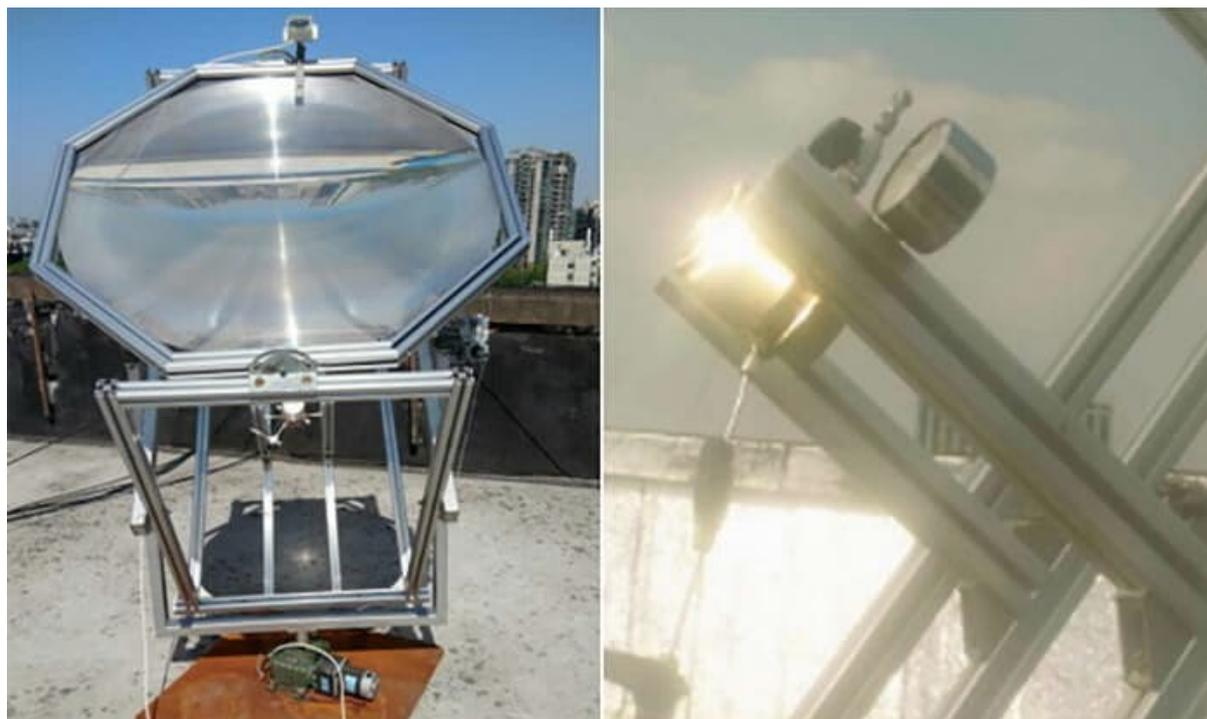
Figure 1.4. Solar concentrator setup for batch photocatalytic CO<sub>2</sub> reduction (left) and close-up of its reaction chamber (right). Reprinted with permission from ref <sup>(52)</sup>. Copyright 2021 AIP Publishing.
