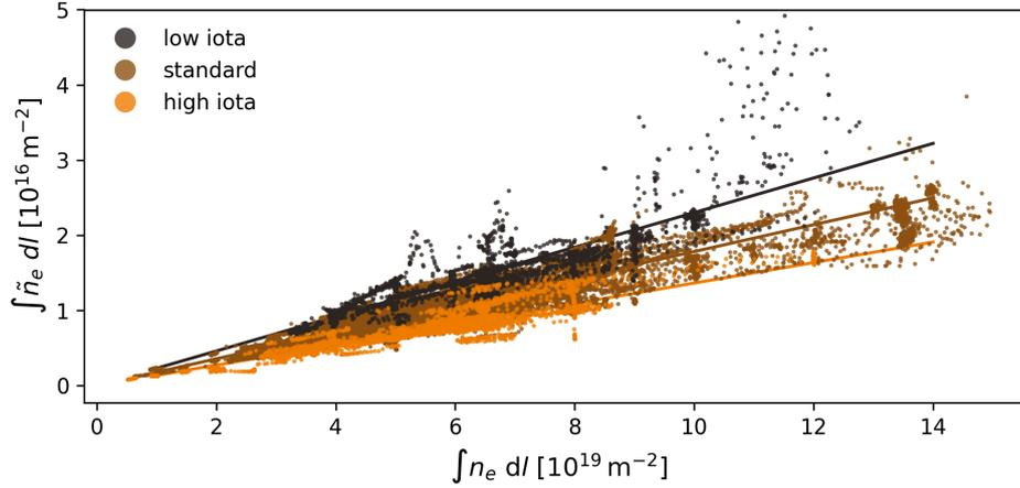
Figure 1: Line-integrated density fluctuation amplitude versus line-integrated density in three magnetic configurations of W7-X with varying rotational transform. Data points represent averages of 100 ms-segments in purely electron-cyclotron-resonance-heated (ECRH) hydrogen plasma with gas-fuelling from the edge. Solid lines represent linear regressions to all data points of one configuration.
