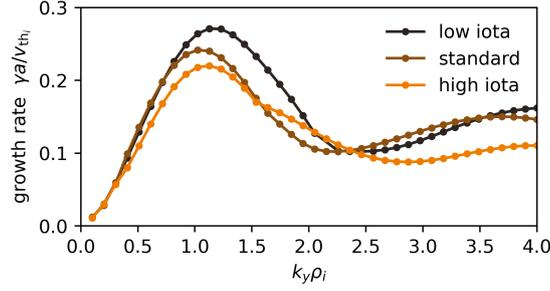
Figure 2: Linear growth rate spectra from gyrokinetic simulations using stella with  $a/L_{T_e} = 0$ . The main ITG peak around  $k_y \rho_i = 1$  shows the same trend as the experimental observations.
